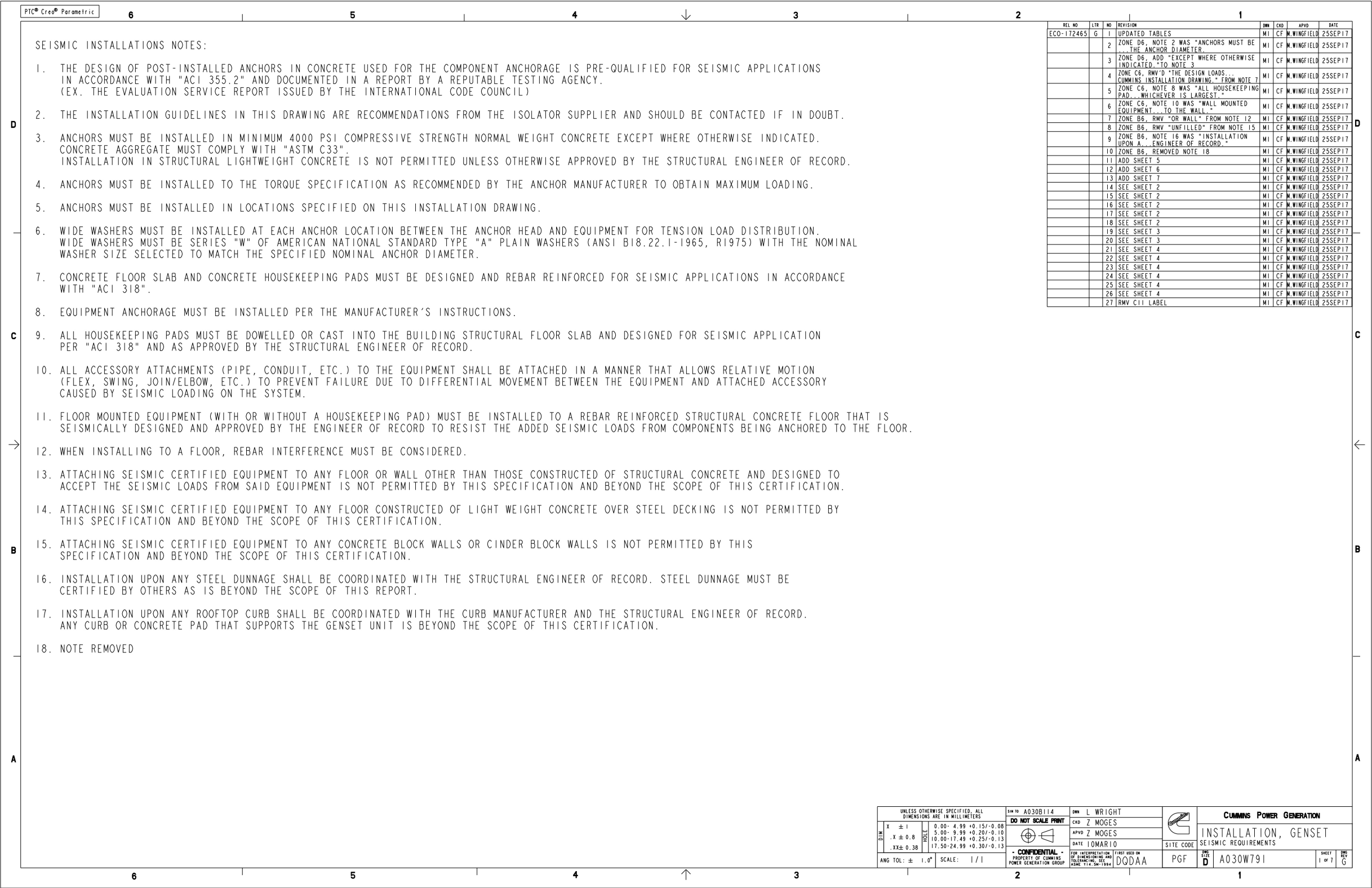
FIGURE 85. SEISMIC INSTALLATION INSTRUCTIONS (SHEET 1 OF 3)
