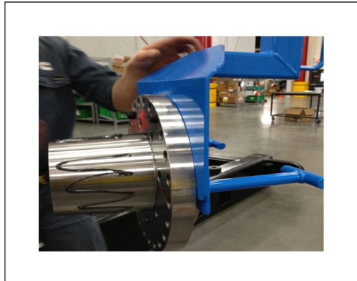
FIGURE 24. LUBRICATE INNER DIAMETER OF THE HUB OUTER RING
