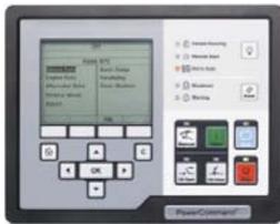
The PowerCommand control system is an integrated microprocessor based generator set control system providing voltage regulation, engine protection, alternator protection, operator interface and isochronous governing.
