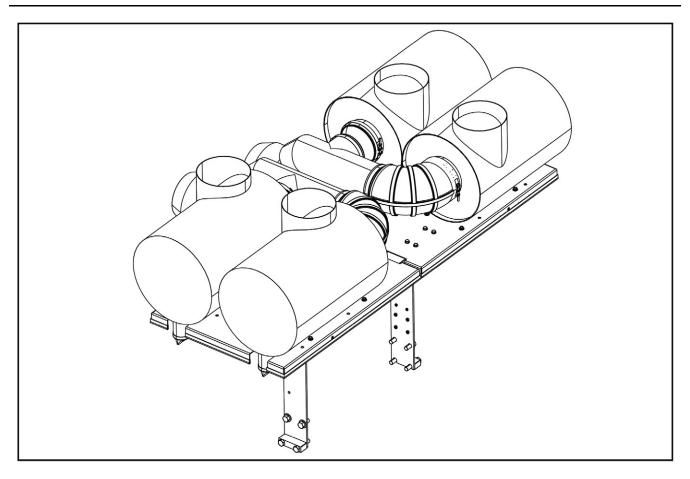
FIGURE 9. HEAVY DUTY AIR CLEANER ASSEMBLY
