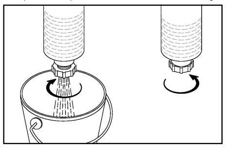
FIGURE 60. DRAINING THE FUEL/WATER SEPARATOR
