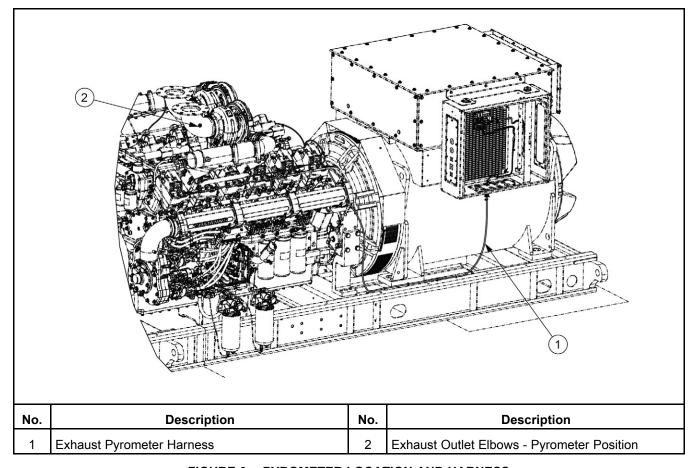
FIGURE 6. PYROMETER LOCATION AND HARNESS
