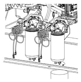
FIGURE 62. DRAINING THE FILTER/SEPARATORS
