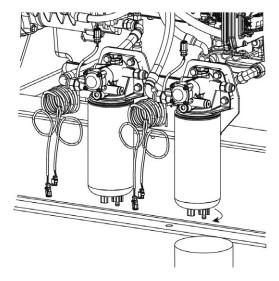
FIGURE 64. FUEL FILTER ELEMENT REPLACEMENT
