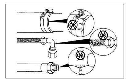
FIGURE 65. HOSES AND FUEL LINE INSPECTION
