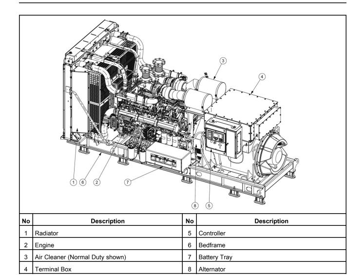
FIGURE 2. TYPICAL QSK38 ENGINE GENERATOR SET
