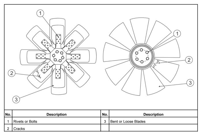
FIGURE 55. COOLING FAN INSPECTION CHECKPOINTS
