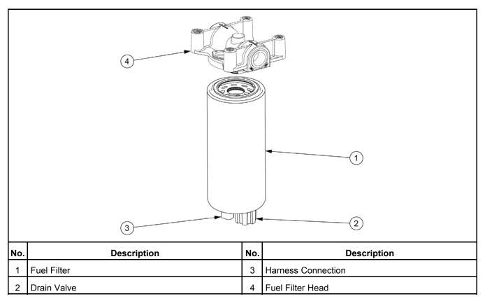
FIGURE 63. FUEL FILTER REMOVAL
