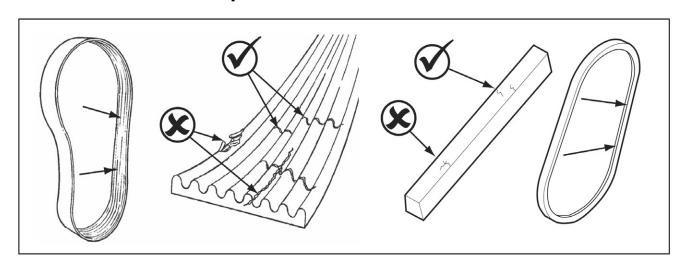
FIGURE 53. DRIVE BELT INSPECTION
