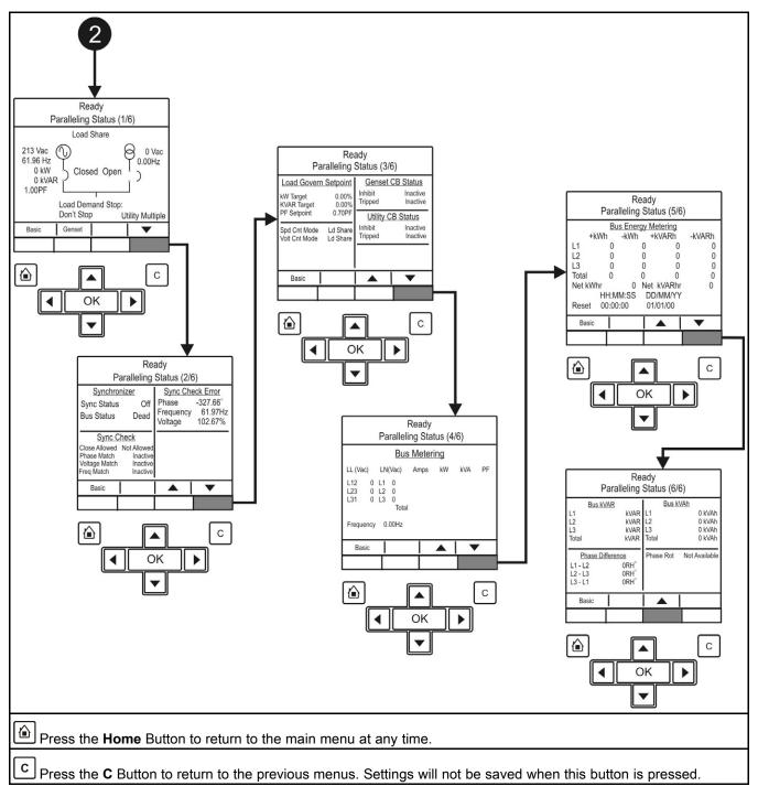
FIGURE 27. PARALLELING STATUS DATA SHEET 2 - TYPICAL DATA
