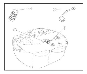
FIGURE 59. TYPICAL OIL SAMPLING VALVE
