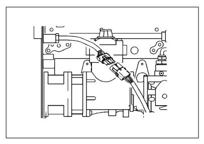
FIGURE 71. CHECK HARNESS CONNECTIONS
