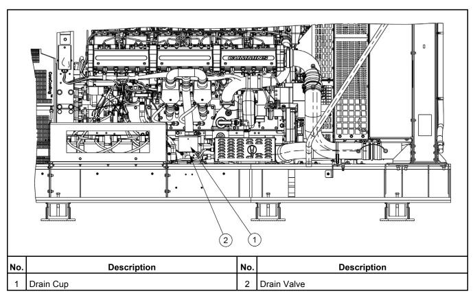
FIGURE 58. CRANKCASE BREATHER OIL DRAIN CUP
