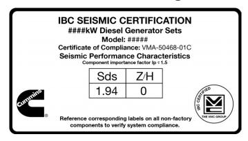
This label indicates that this generator set is IBC compliant.
