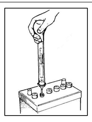
FIGURE 72. CHECKING SPECIFIC GRAVITY
