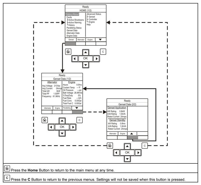
FIGURE 16. GENERATOR SET DATA MENU - TYPICAL DATA
