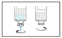
FIGURE 61. DRAINING THE FUEL/WATER-SEPARATOR
