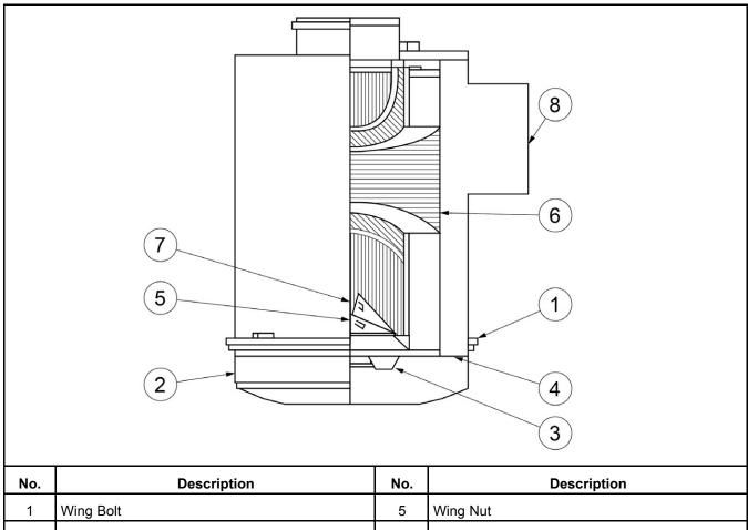
No.DescriptionNo.Description1Wing Bolt5Wing Nut2Air Filter Cap6Air Cleaner Primary Element3Wing Nut7Wing Nut4Dust Shield8Dust Pan
