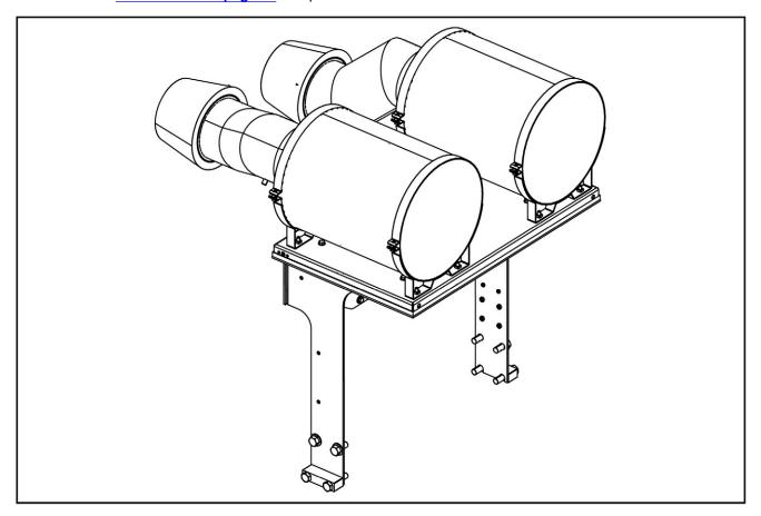
FIGURE 8. NORMAL AIR CLEANER ASSEMBLY
