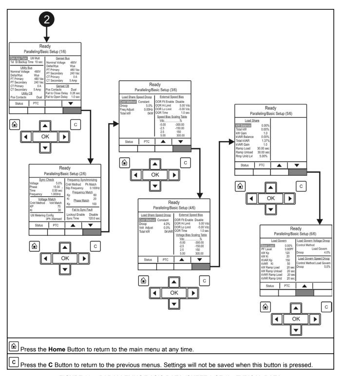
FIGURE 29. PARALLELING/BASIC DATA (SHEET 2 OF 2) - TYPICAL DATA
