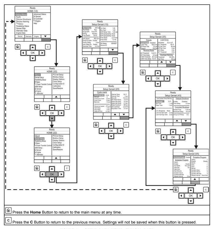
FIGURE 25. SETUP DATA MENU - TYPICAL DATA
