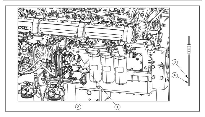
FIGURE 56. OIL LEVEL CHECK
