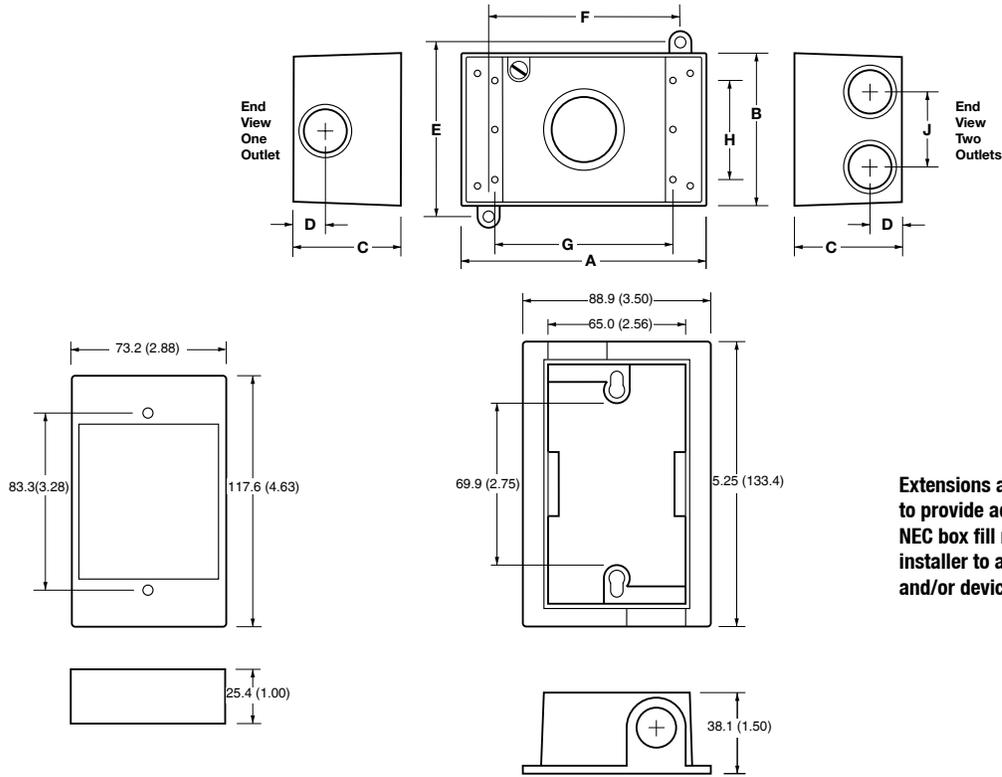
Extensions and Extension Adapters are used to provide additional capacity needed for NEC box fill requirements. Adapters allow installer to add "takeoffs" to new boxes and/or devices.
