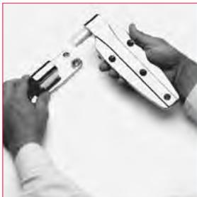
3. Reposition strap into flange and replace cap.
