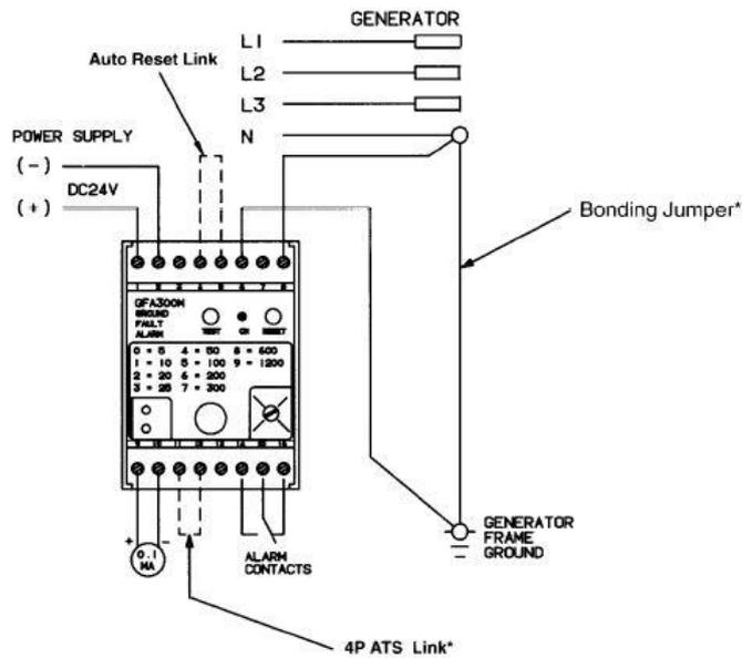
\* Required only with separately derived systems. Bonding jumper is included in kit.
