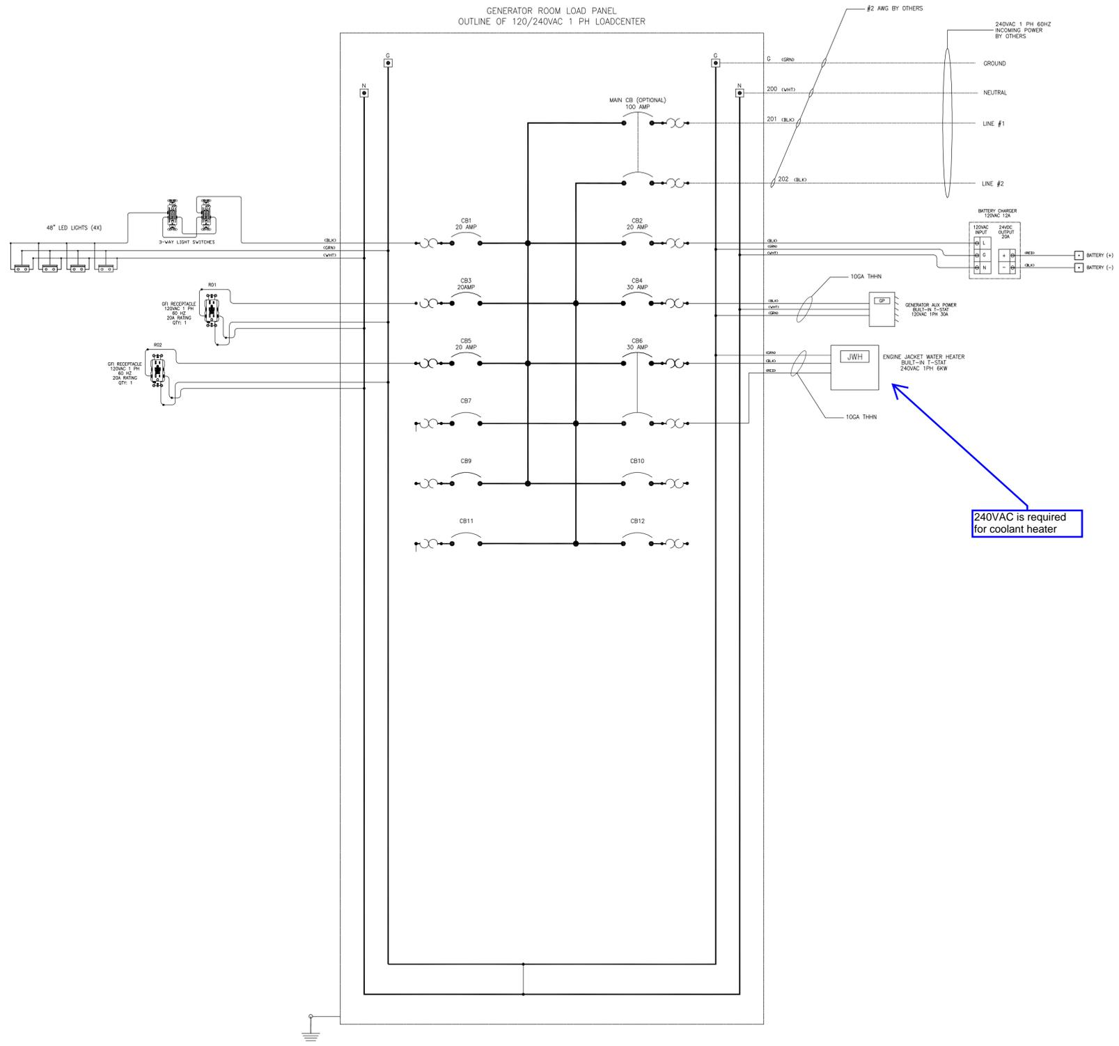
240VAC is required for coolant heater
