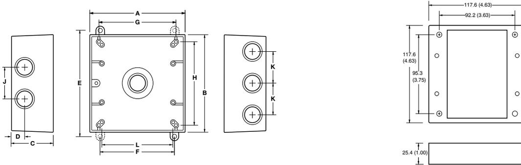
**Extension WE2 – Dimensions in Millimeters (Inches) Extensions and Extension Adapters are used to provide additional capacity needed for NEC box fill requirements. Adapters allow installer to add “take-offs” to new boxes and/or devices.**
