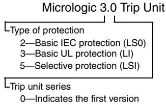
Micrologic trip units are field replaceable to allow for upgrading of the trip unit in the field. For complete information on available circuit breaker models, frame sizes, interrupting ratings, sensor plugs, rating plugs and trip units, see the product catalog.
