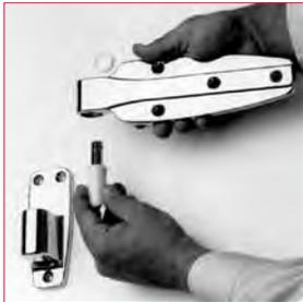
2. Pop out cap. Turn strap 180°, reinsert pin assembly in strap.
