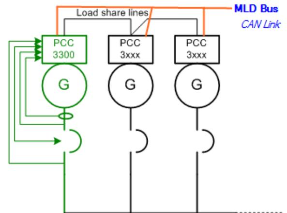
**PCC3300 External Voltage and Frequency Biasing Inputs**
