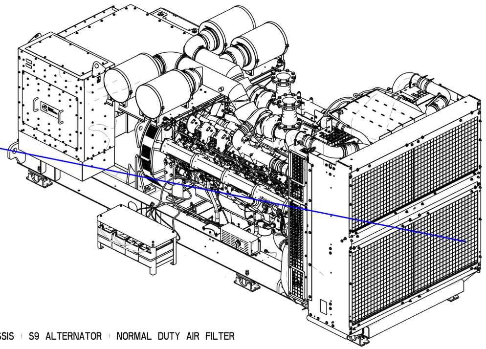
HARD MOUNTED CHASSIS + S9 ALTERNATOR + NORMAL DUTY AIR FILTER
