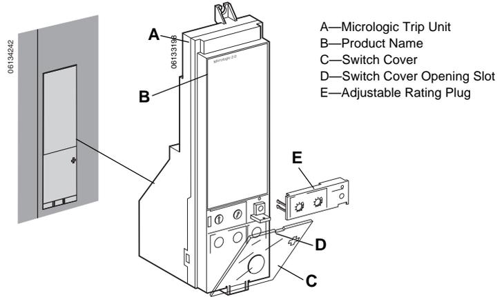
On the face of the trip unit are adjustable switches to allow changing of trip characteristics. Trip units are shipped with the long-time pickup switch set at 1.0 and all other trip unit adjustments set at their lowest settings.
