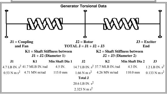
Engine: C7.1Generator Frame: LC5034HGenset Rating (kW): 200.0Line Voltage: 480Fuel: DieselGenerator Arrangement: 3544073Genset Rating (kVA): 250.0Phase Voltage: 277Frequency: 60Excitation Type: Permanent MagnetPwr. Factor: 0.8Rated Current: 300.7
