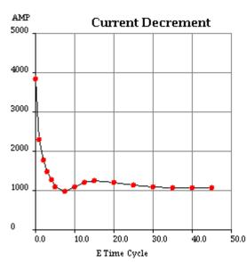
Instantaneous 3 Phase Fault Current: 3839 Amps Instantaneous Line - Line Fault Current: 3148 Amps Instantaneous Line - Neutral Fault Current: 5313 Amps
