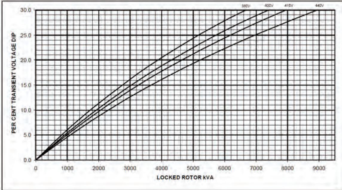
Locked Rotor Motor Starting Curve
