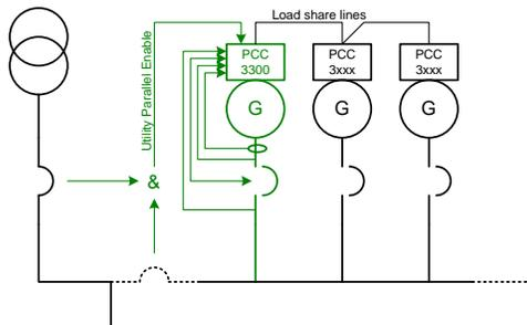
**Power Transfer Control:** Control operates a single genset/single utility transfer pair in open transition, fast closed transition, or soft closed transition. Extended paralleling functionality also provides base load and peak shave options.
