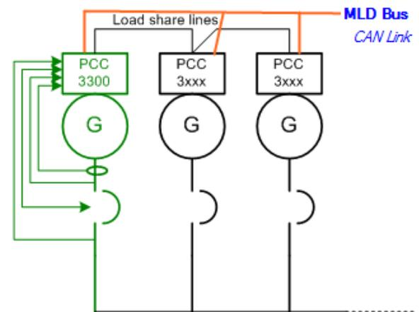
**PCC3300 External Voltage and Frequency Biasing Inputs**
