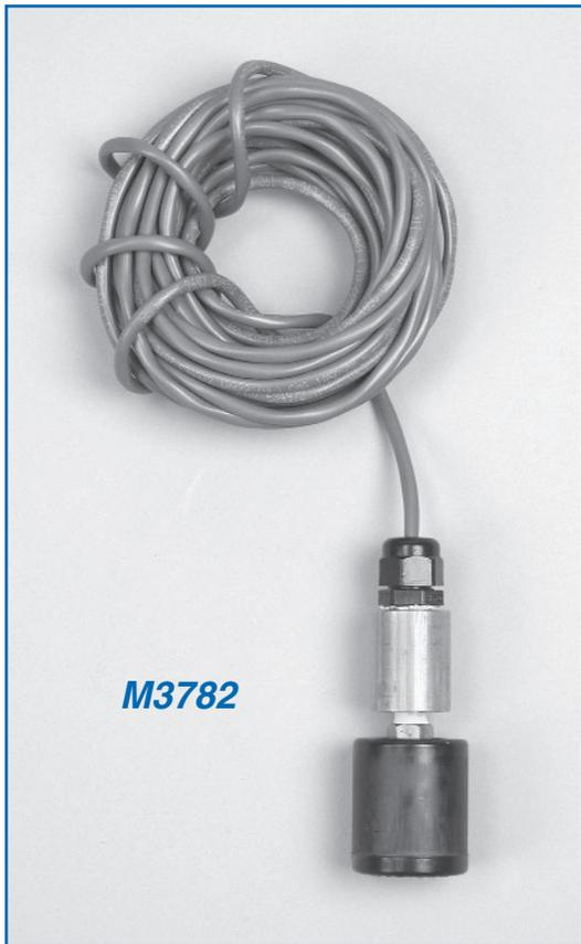
Madison Company offers a standard model M3782 liquid level switch that can be fully submerged with 20' of 22 AWG HALAR® jacketed 2-conductor wire. This model is weighted for suspension in non-magnetic tanks and can be used in conjunction with a still pipe. Its materials are suitable for water, hydrocarbons and certain chemicals. Contact Madison Company to check on material compatibility.
