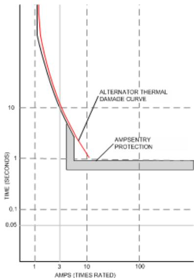
AmpSentry Maintenance Mode (AMM) - Instantaneous tripping, if AmpSentry Maintenance mode is active (50mS response to turn off AVR excitation/shutdown genset) for arc flash reduction when personnel are near genset.
