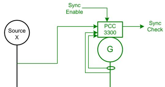
Isolated Bus: allows the genset to perform a dead bus closure or synchronize to the bus and isochronously share kW and kVAR loads with other gensets.
