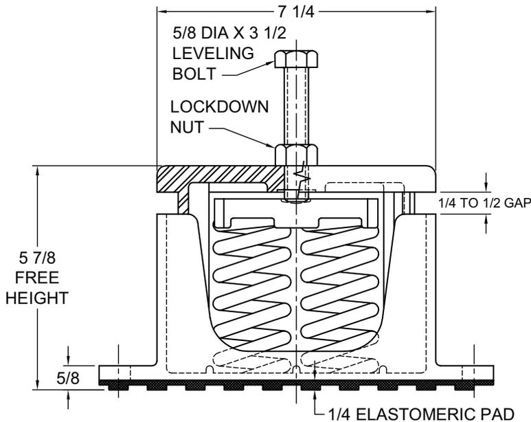
**TYPE C4E-1D CAST IRON SPRING-FLEX MOUNTINGS WITH EXTERNAL ADJUSTMENT**
