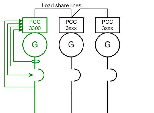
**Utility Single:** Control monitors one genset and utility. The control will automatically start and provide power to a load if the utility fails. The control will also resynchronize the genset back to the utility and provides extended paralleling capabilities.
