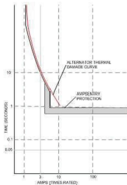
AmpSentry Maintenance Mode (AMM) - Instantaneous tripping, if AmpSentry Maintenance mode is active (50mS response to turn off AVR excitation/shutdown genset) for arc flash reduction when personnel are near genset.
