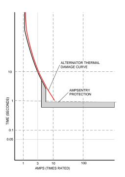
**Over current warning** - Output current on any phase at more than 110% of rating for more than 60 seconds.
