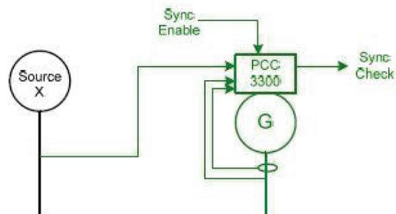
**Isolated Bus:** allows the genset to perform a dead bus closure or synchronize to the bus and isochronously share kW and kVAR loads with other gensets.
