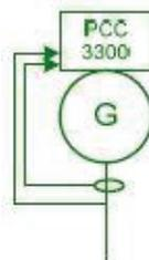
**Synchronizer only:** control will synchronize the genset to other source when commanded to either via a hardwired or Modbus driven input.
