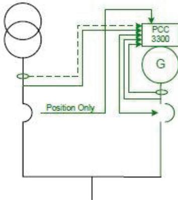
**Utility multiple:** Supports all functionality of Isolated Bus and provides extended paralleling to the utility. Extended paralleling load set points follow a constant setting; dynamically follow an analog input, ModBus register or HMI.
