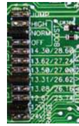
Field selectable jumper
