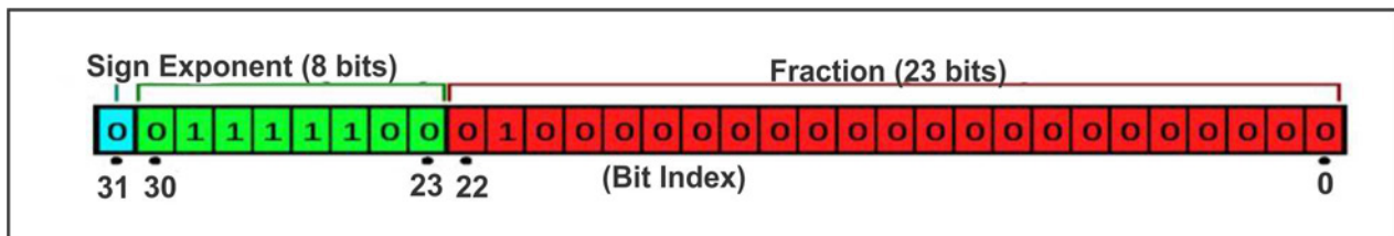
FIGURE 1. BIT FORMAT FOR IEEE 754
