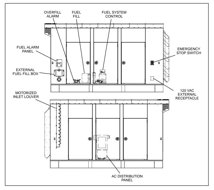
FIGURE 7-1. OPTIONAL ENCLOSURE FEATURES (WEATHER ENCLOSURE SHOWN)
