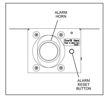
FIGURE 7-2. OVERFILL ALARM PANEL
