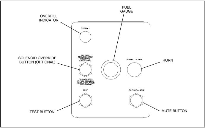
FIGURE 5-6. EXTERNAL ALARM PANEL
