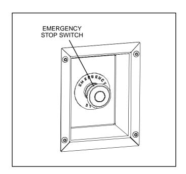
FIGURE 7-3. EXTERNAL EMERGENCY STOP SWITCH
