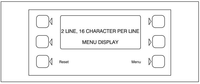
FIGURE 3-2. DIGITAL DISPLAY AND MENU SELECTION SWITCHES
