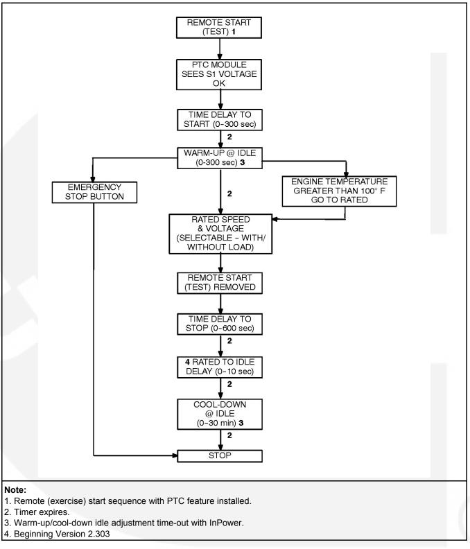
FIGURE 17. PTC FEATURE REMOTE START TEST/EXERCISE SWITCH - AUTO MODE
