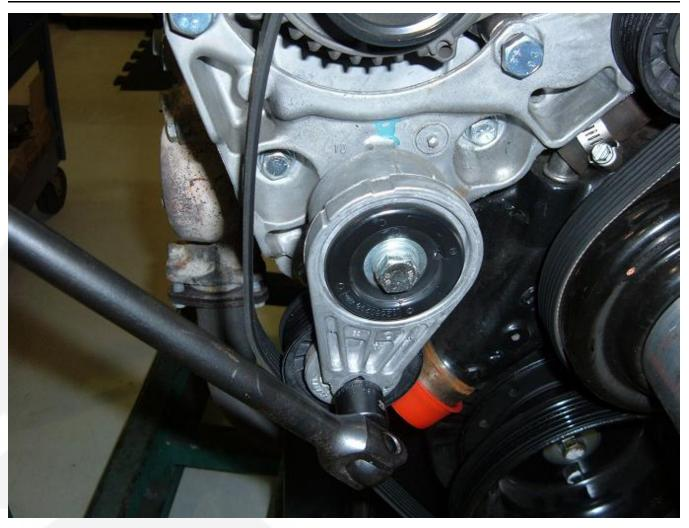
FIGURE 28. BELT REPLACEMENT WITH RATCHET INSERTED IN TENSIONER
