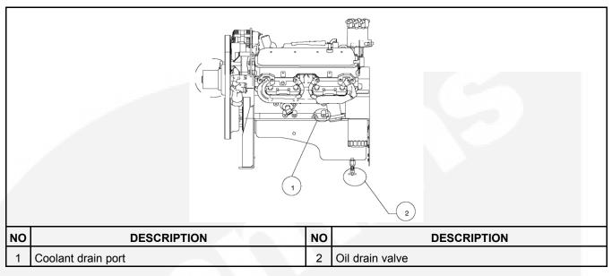
FIGURE 25. DRAIN PORTS LOCATIONS FOR ENGINE OIL AND COOLANT
