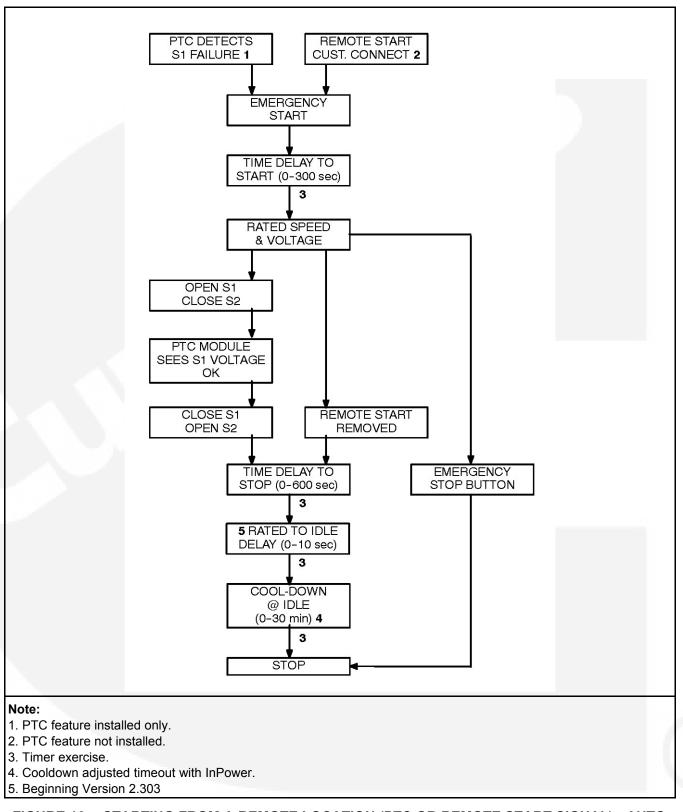
FIGURE 16. STARTING FROM A REMOTE LOCATION (PTC OR REMOTE START SIGNAL) - AUTO MODE
