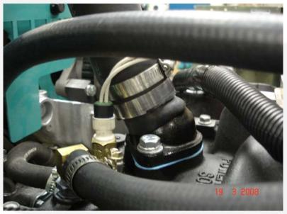
FIGURE 22. LP VAPORIZER ON ENGINE (IF USED)
