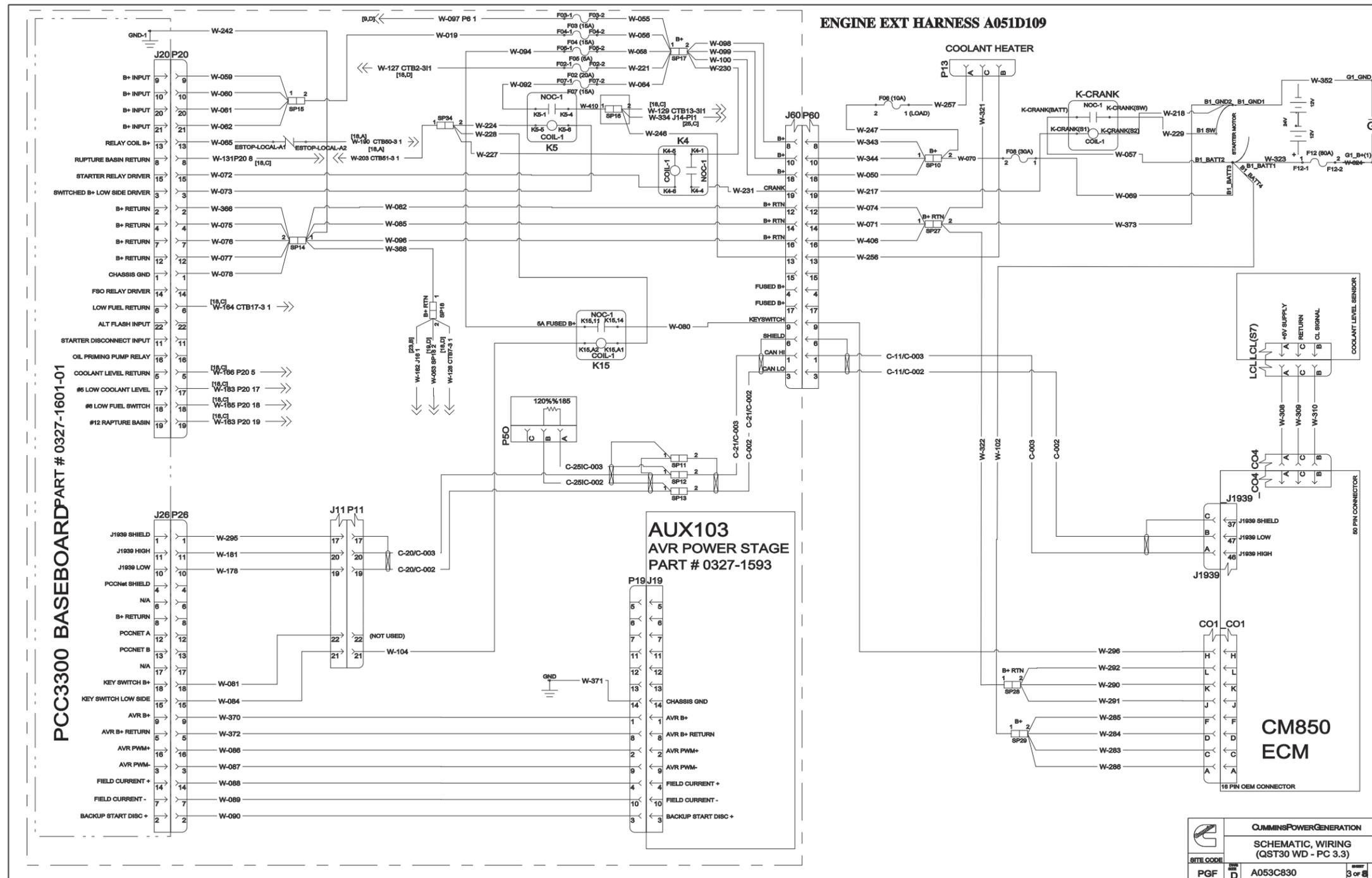
FIGURE 82. ENGINE EXTENSION HARNESS - WIRING DIAGRAM
