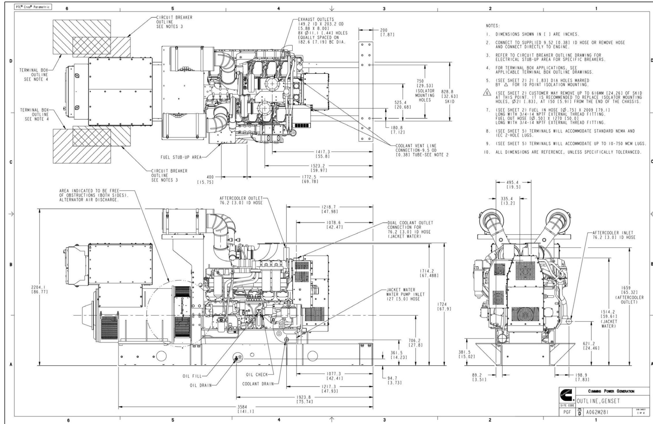
FIGURE 76. GENERATOR SET OUTLINE DRAWING (REMOTE RADIATOR) (SHEET 1)
