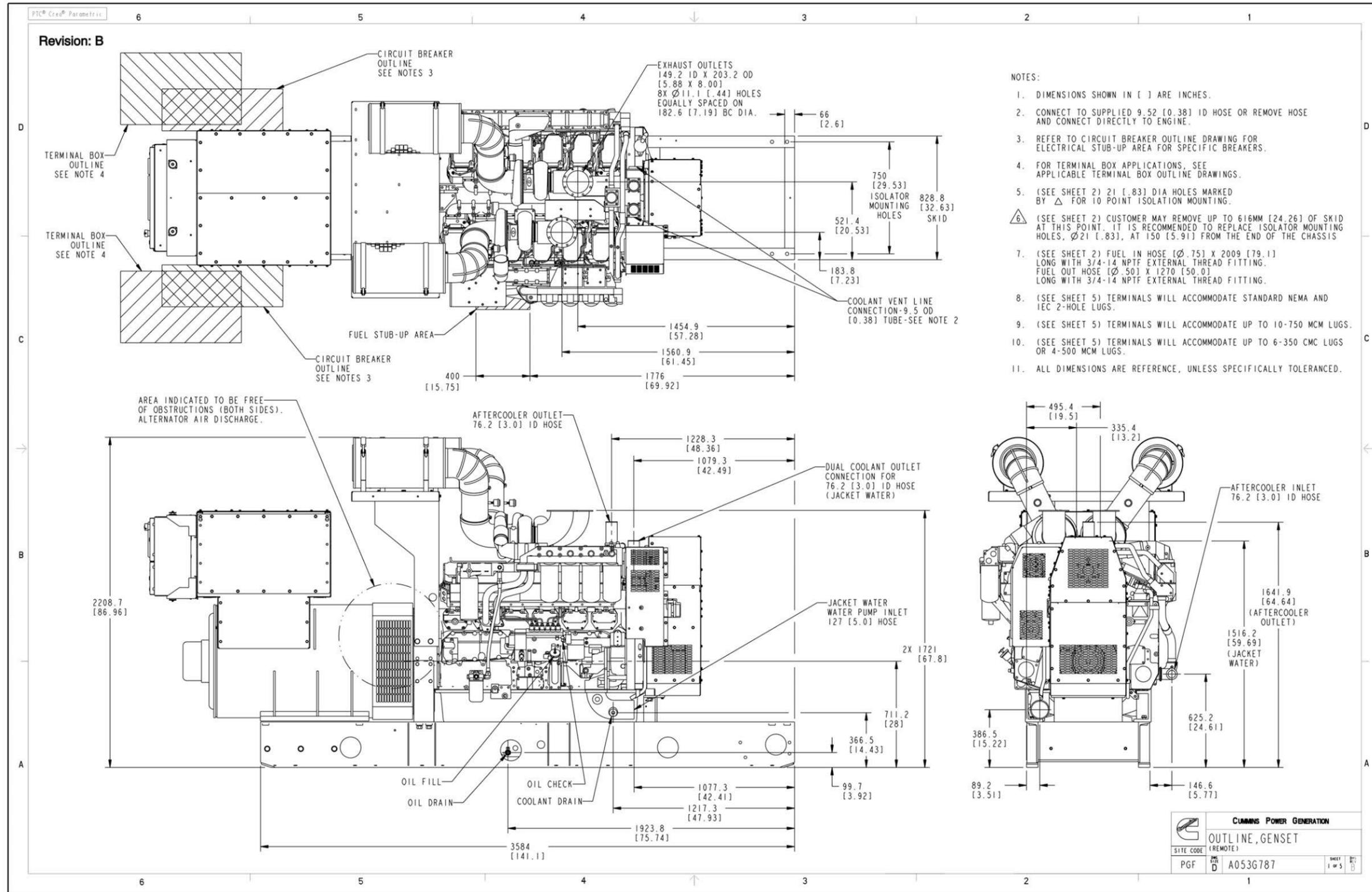
FIGURE 71. GENERATOR SET OUTLINE DRAWING (REMOTE RADIATOR) (SHEET 1)
