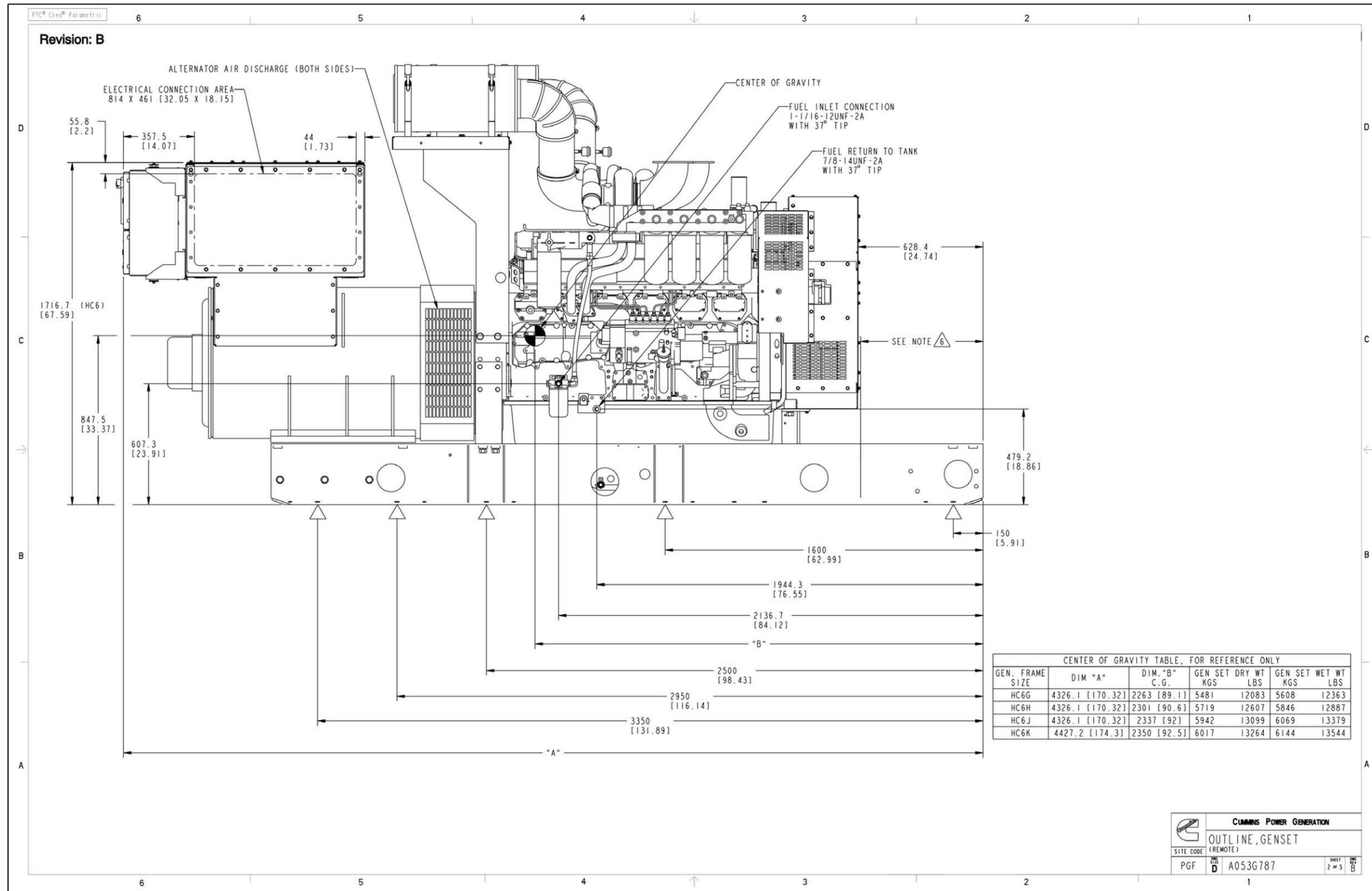
FIGURE 72. GENERATOR SET OUTLINE DRAWING (REMOTE RADIATOR) (SHEET 2)
