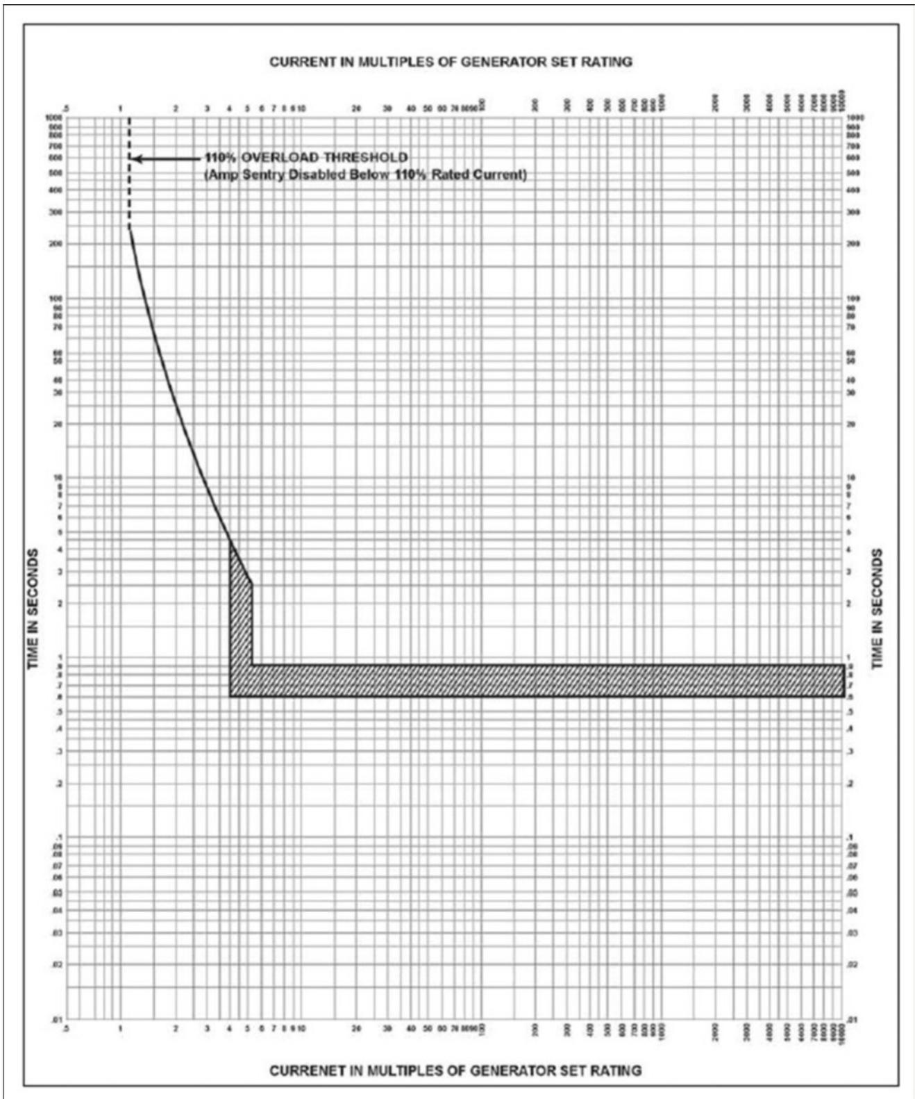
FIGURE 20. AMPSENTRY PROTECTIVE RELAY TIME OVER-CURRENT CHARACTERISTIC CURVE
