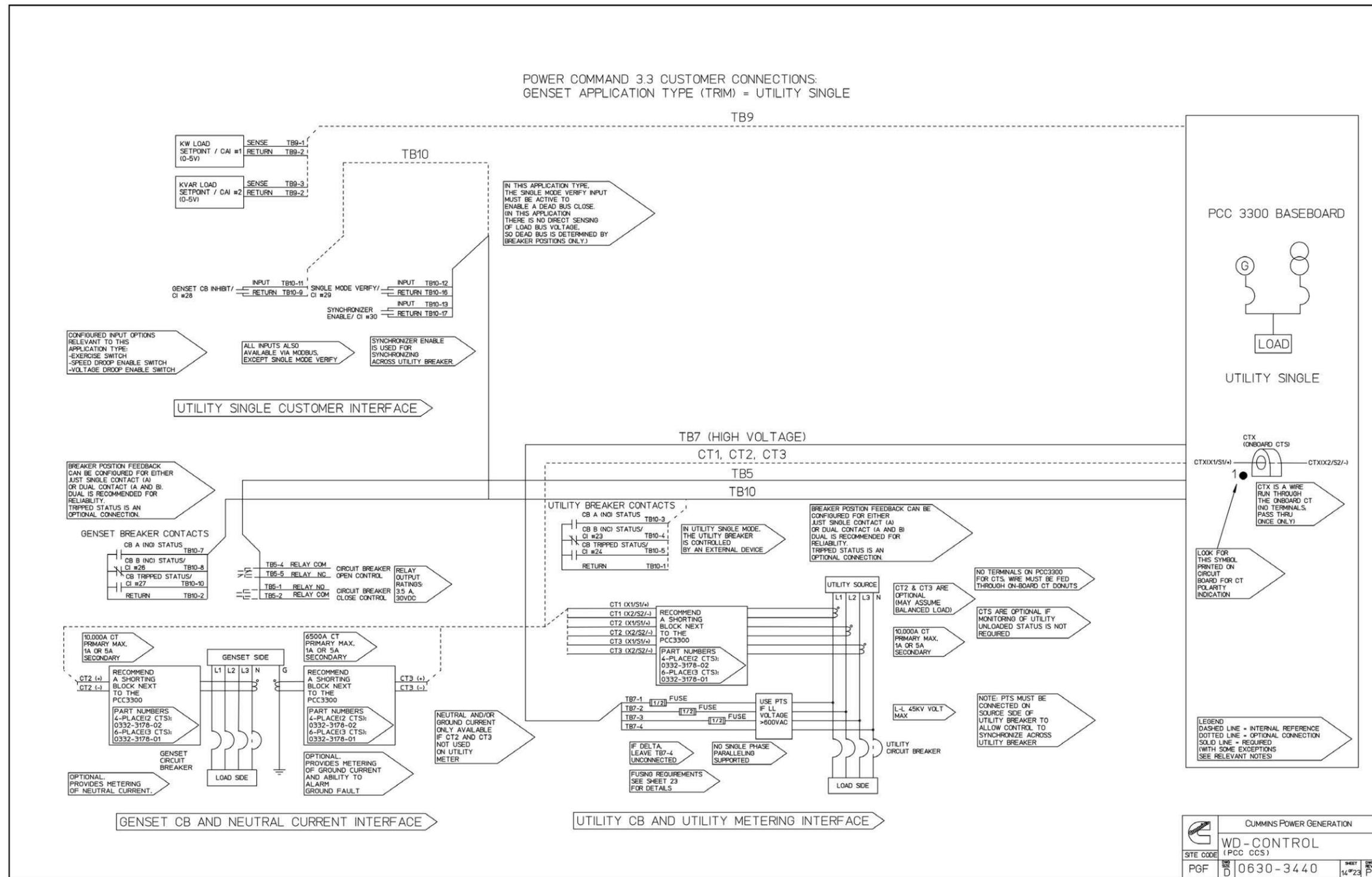
FIGURE 55. POWERCOMMAND 3.3 PARALLELING CONNECTIONS - UTILITY SINGLE
