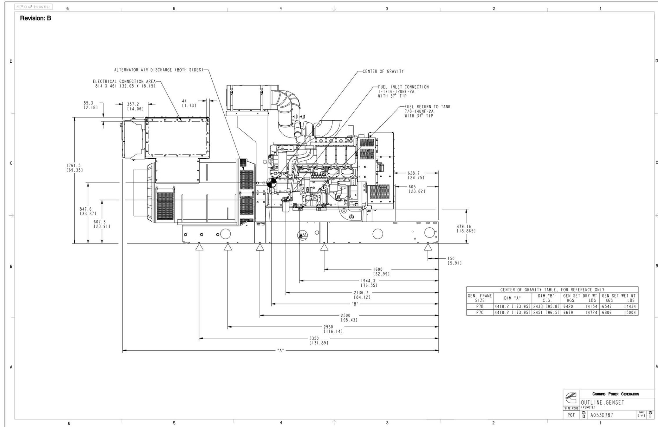
FIGURE 73. GENERATOR SET OUTLINE DRAWING (REMOTE RADIATOR) (SHEET 3)
