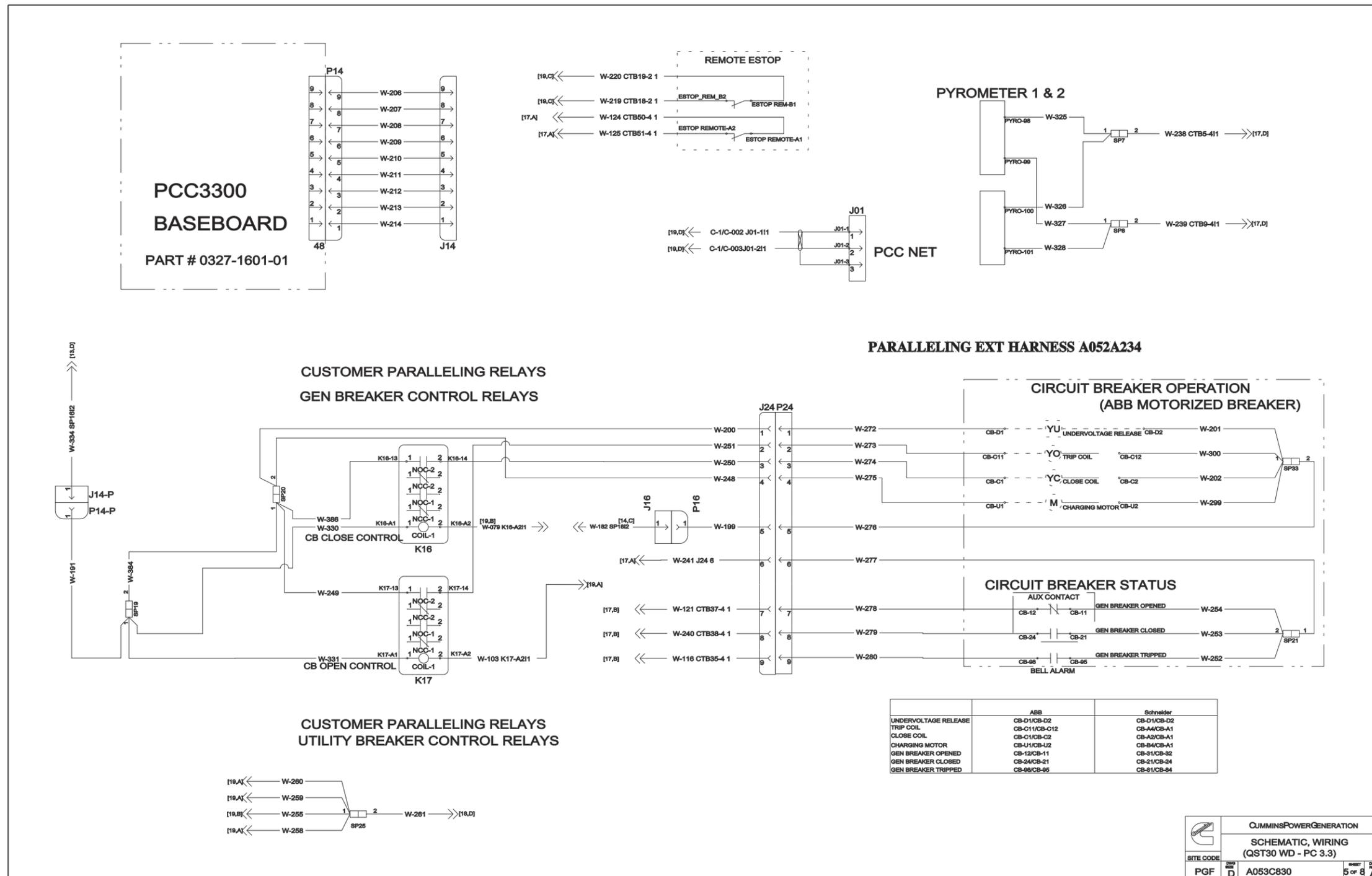
FIGURE 84. AUX 101, AUX 102 - WIRING DIAGRAM
