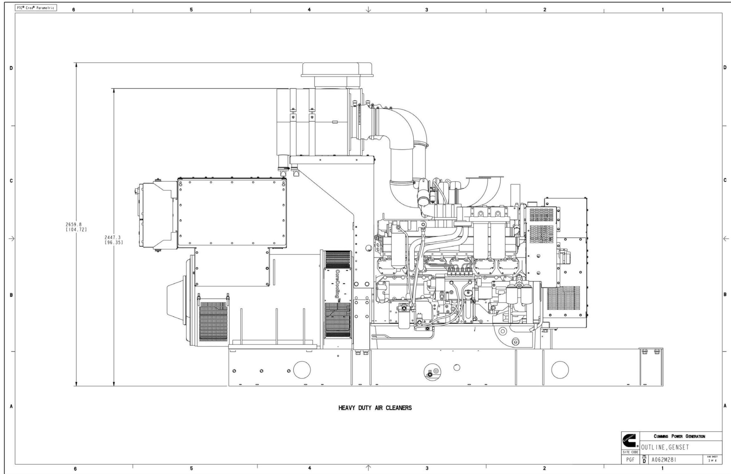
FIGURE 78. GENERATOR SET OUTLINE DRAWING (REMOTE RADIATOR) (SHEET 3)
