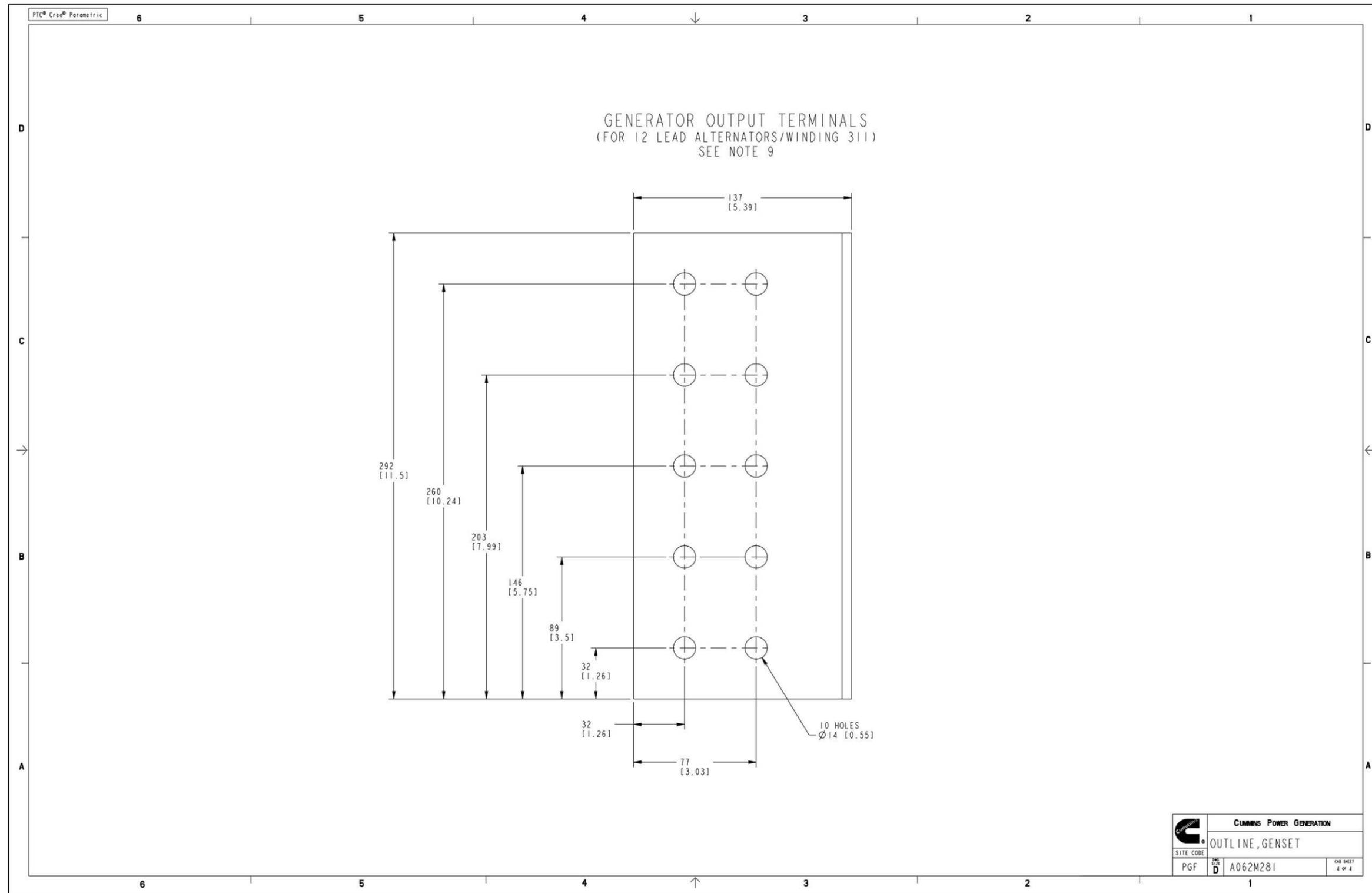
FIGURE 79. GENERATOR SET OUTLINE DRAWING (REMOTE RADIATOR) (SHEET 4)
