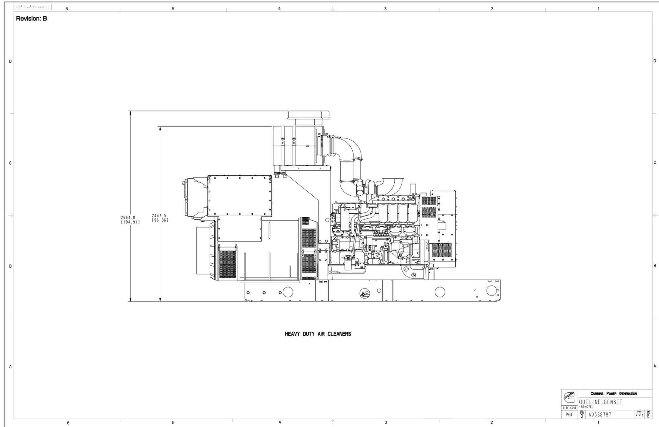
FIGURE 74. GENERATOR SET OUTLINE DRAWING (REMOTE RADIATOR) (SHEET 4)
