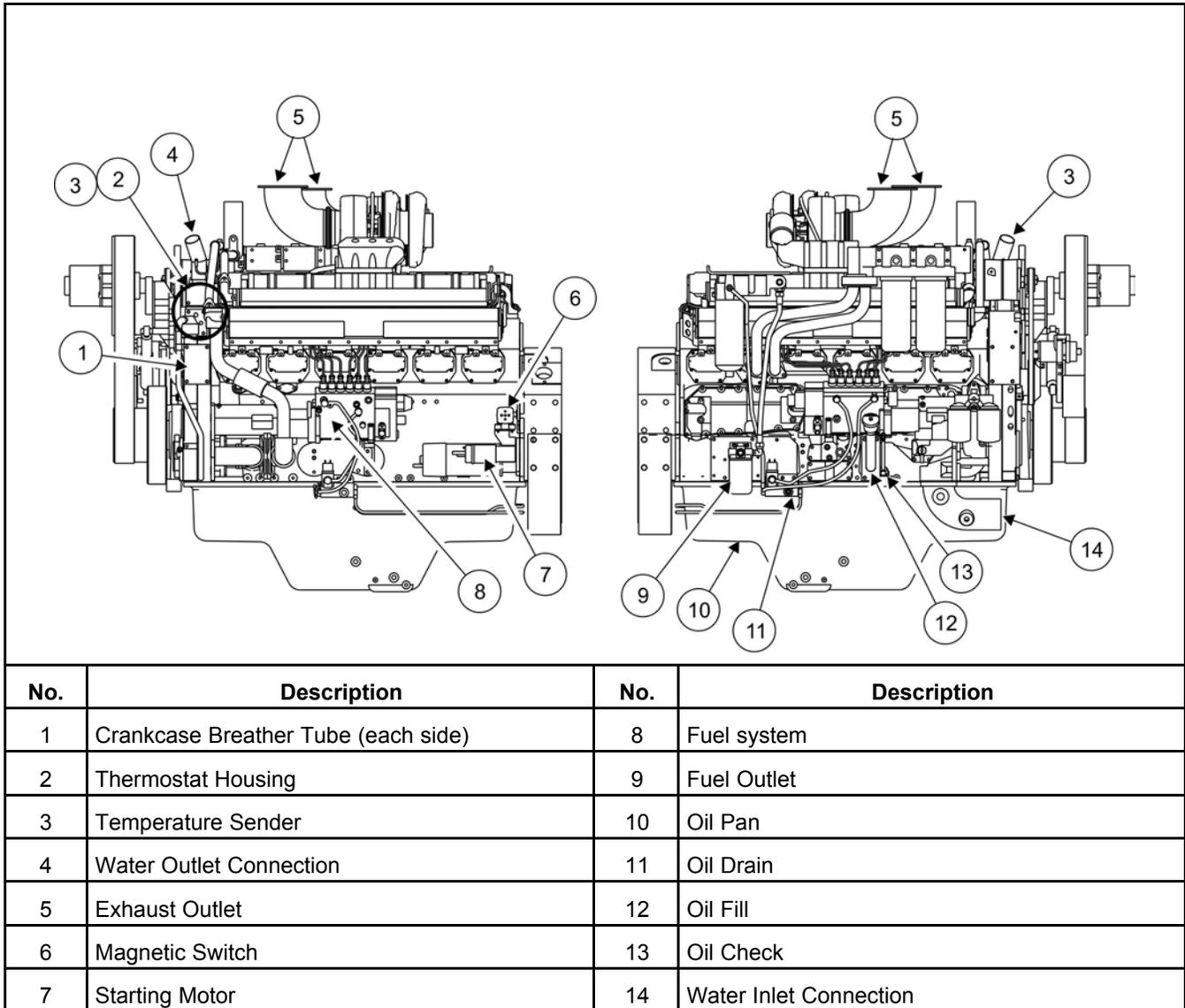
FIGURE 3. ENGINE COMPONENTS
