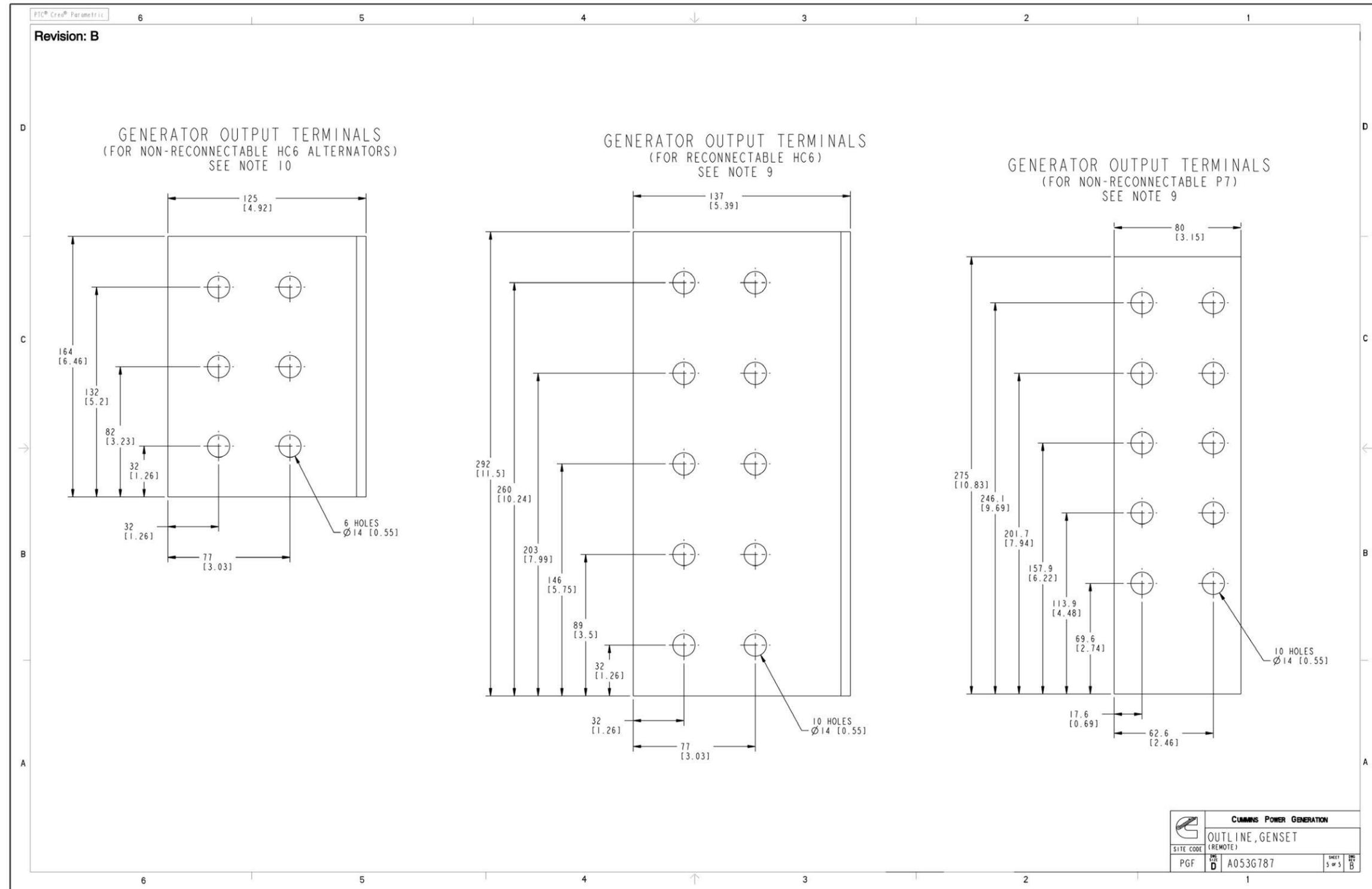
FIGURE 75. GENERATOR SET OUTLINE DRAWING (REMOTE RADIATOR) (SHEET 5)
