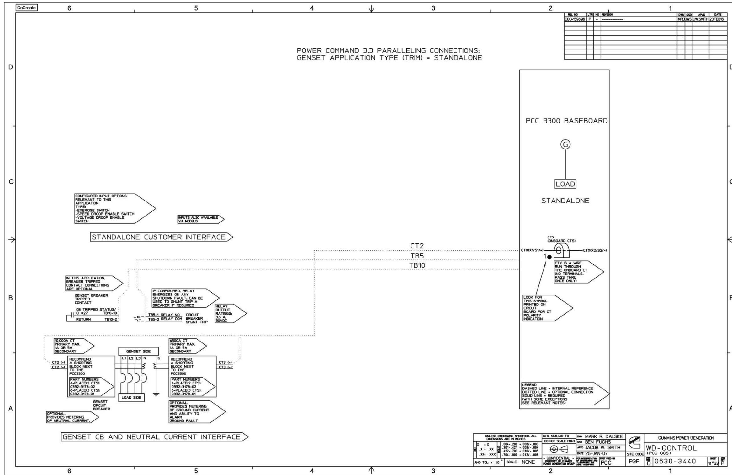
FIGURE 52. POWERCOMMAND 3.3 PARALLELING CONNECTIONS - STANDALONE GENERATOR SET
