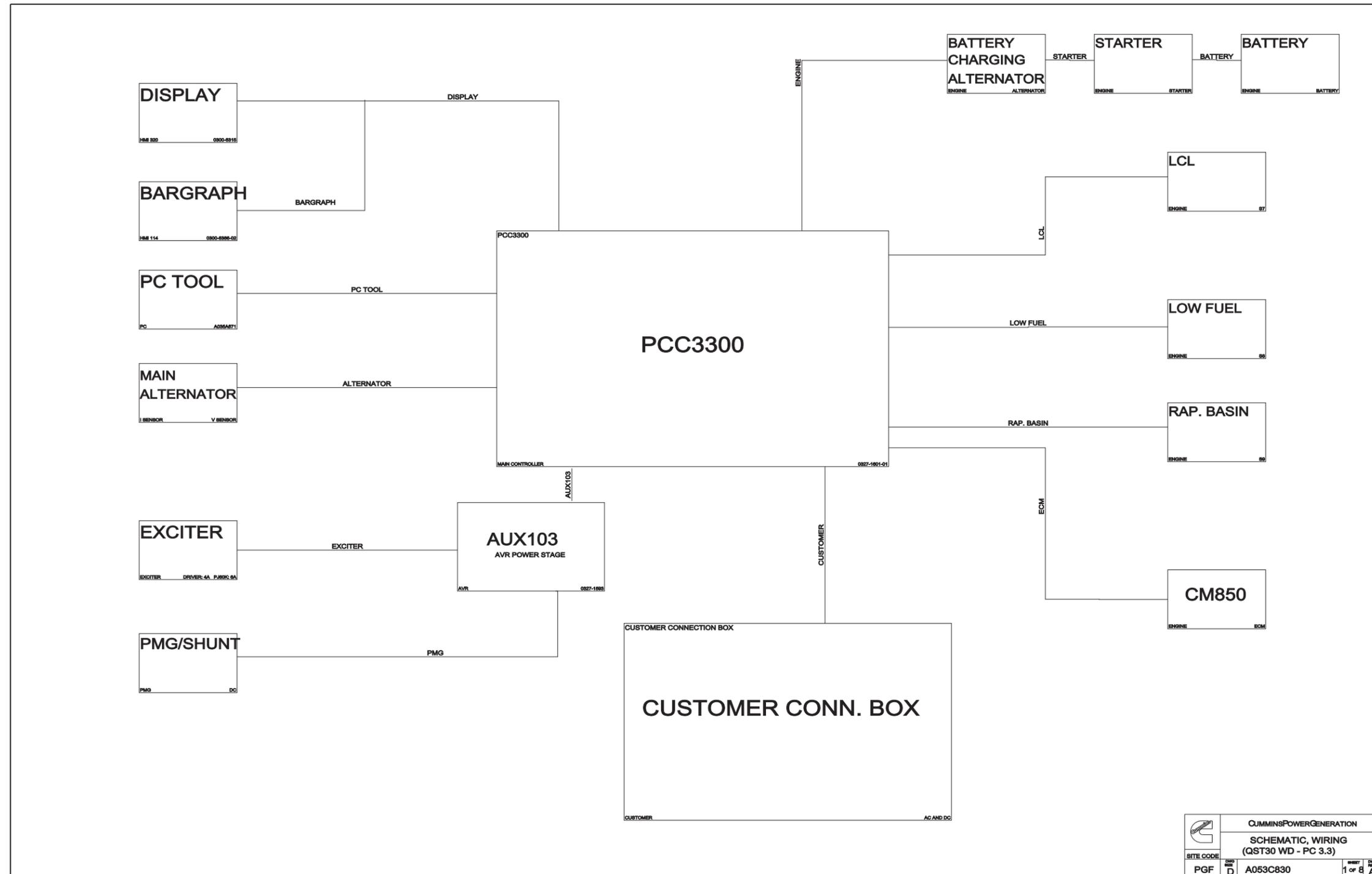
FIGURE 80. PC 3.3 SCHEMATIC
