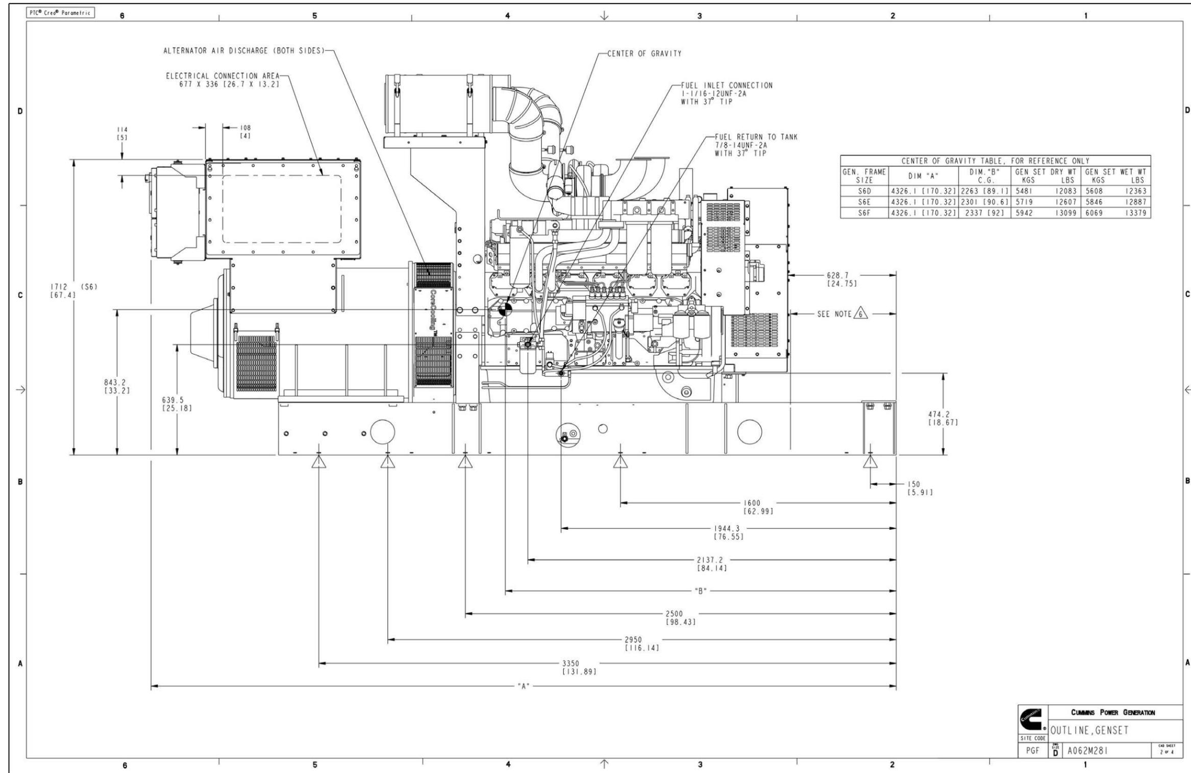
FIGURE 77. GENERATOR SET OUTLINE DRAWING (REMOTE RADIATOR) (SHEET 2)
