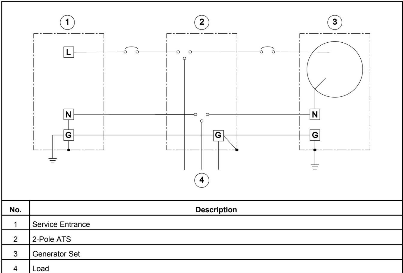
**FIGURE 29. TYPICAL SYSTEM - ONE-PHASE, THREE WIRE UTILITY, TWO-POLE ATS**
