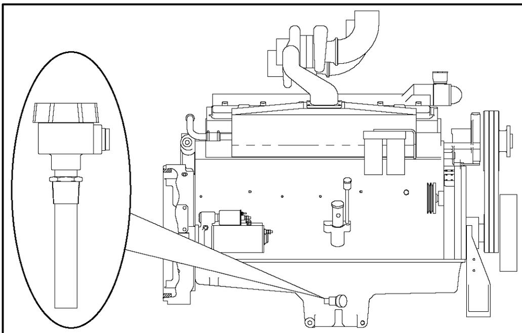
**FIGURE 6. OIL PAN HEATER USED IN 480V APPLICATIONS**
