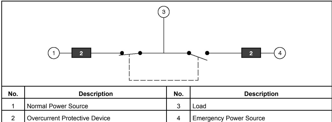
FIGURE 22. TYPICAL LOAD TRANSFER FUNCTION
