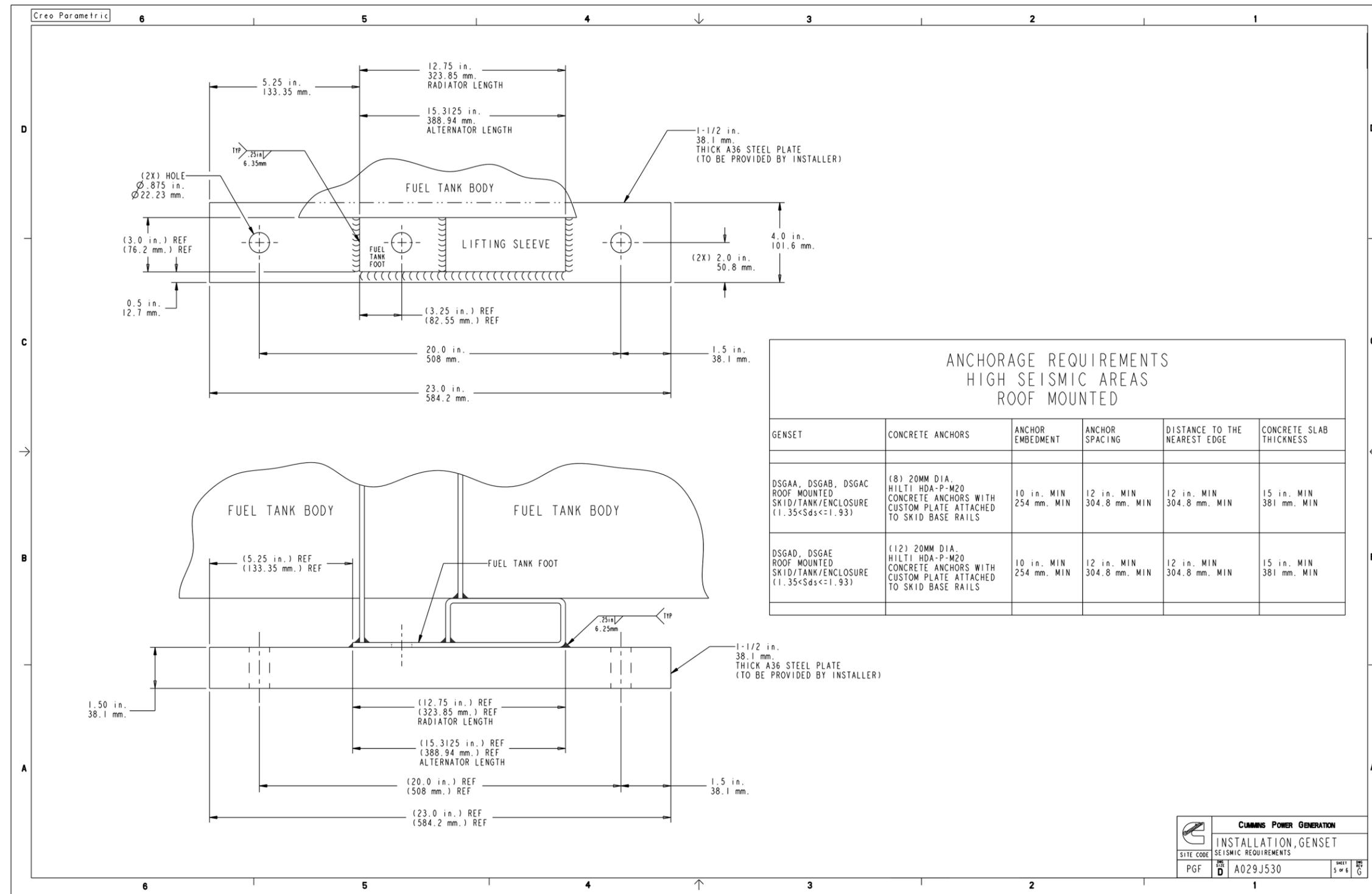
FIGURE 47. SEISMIC INSTALLATION INSTRUCTIONS (SHEET 5 OF 5)
