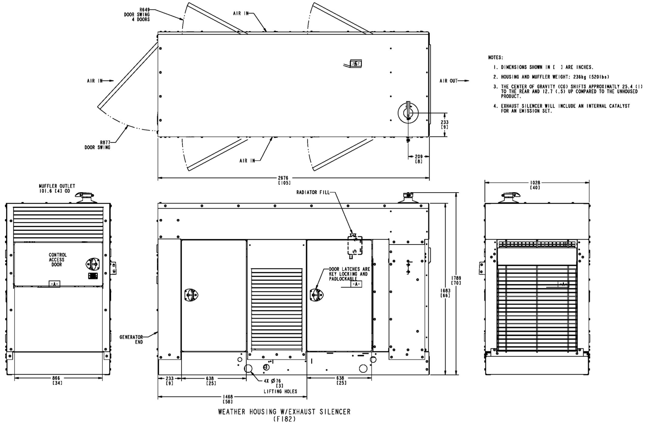
FIGURE 38. OUTLINE DRAWING - WEATHER HOUSED WITH EXHAUST (F182)
