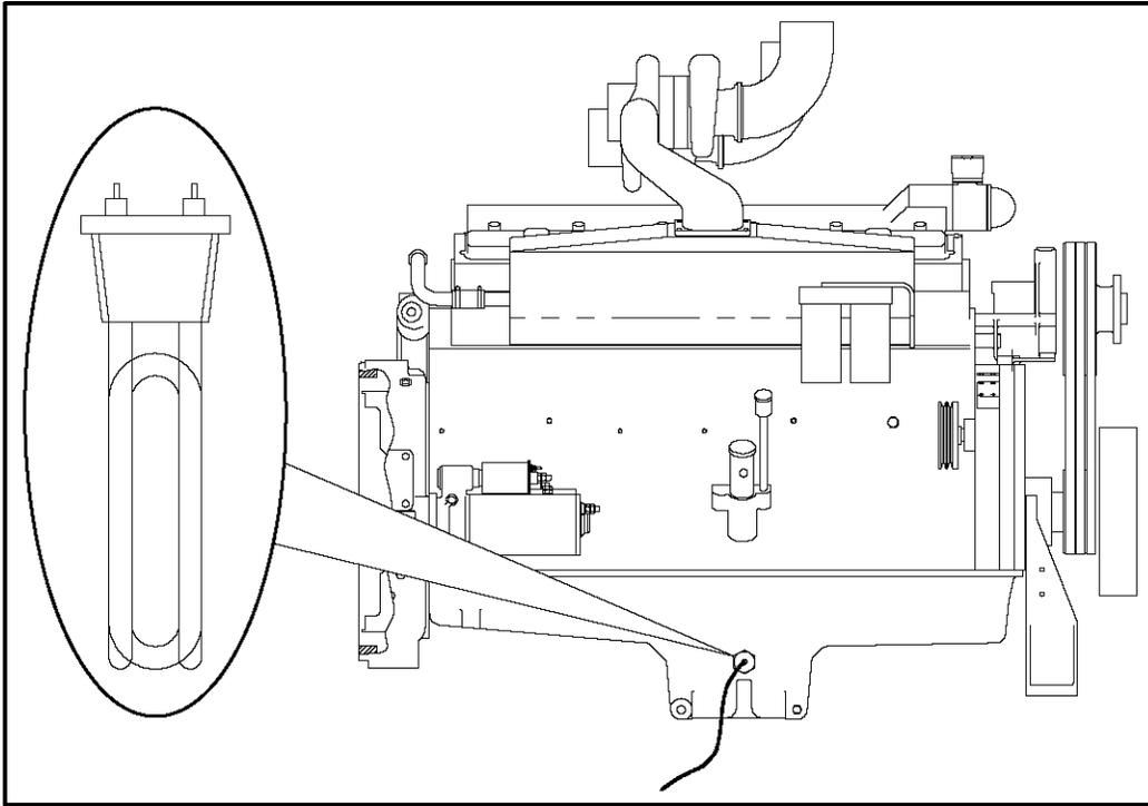
**FIGURE 26. OIL PAN HEATER USED IN 120V AND 208/240V APPLICATIONS**
