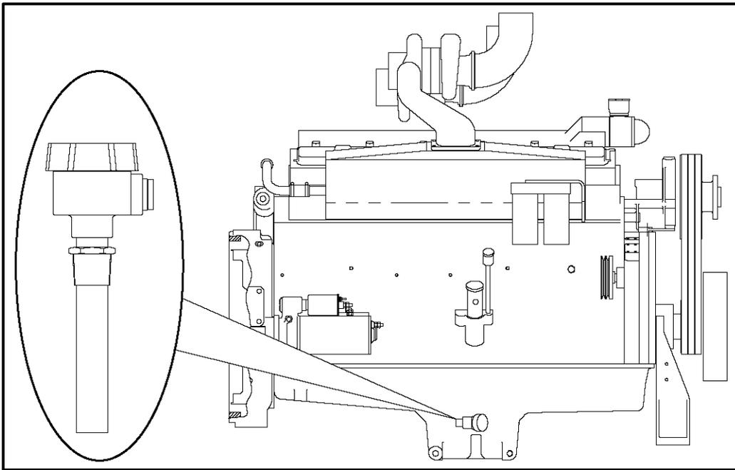
**FIGURE 27. OIL PAN HEATER USED IN 480V APPLICATIONS**
