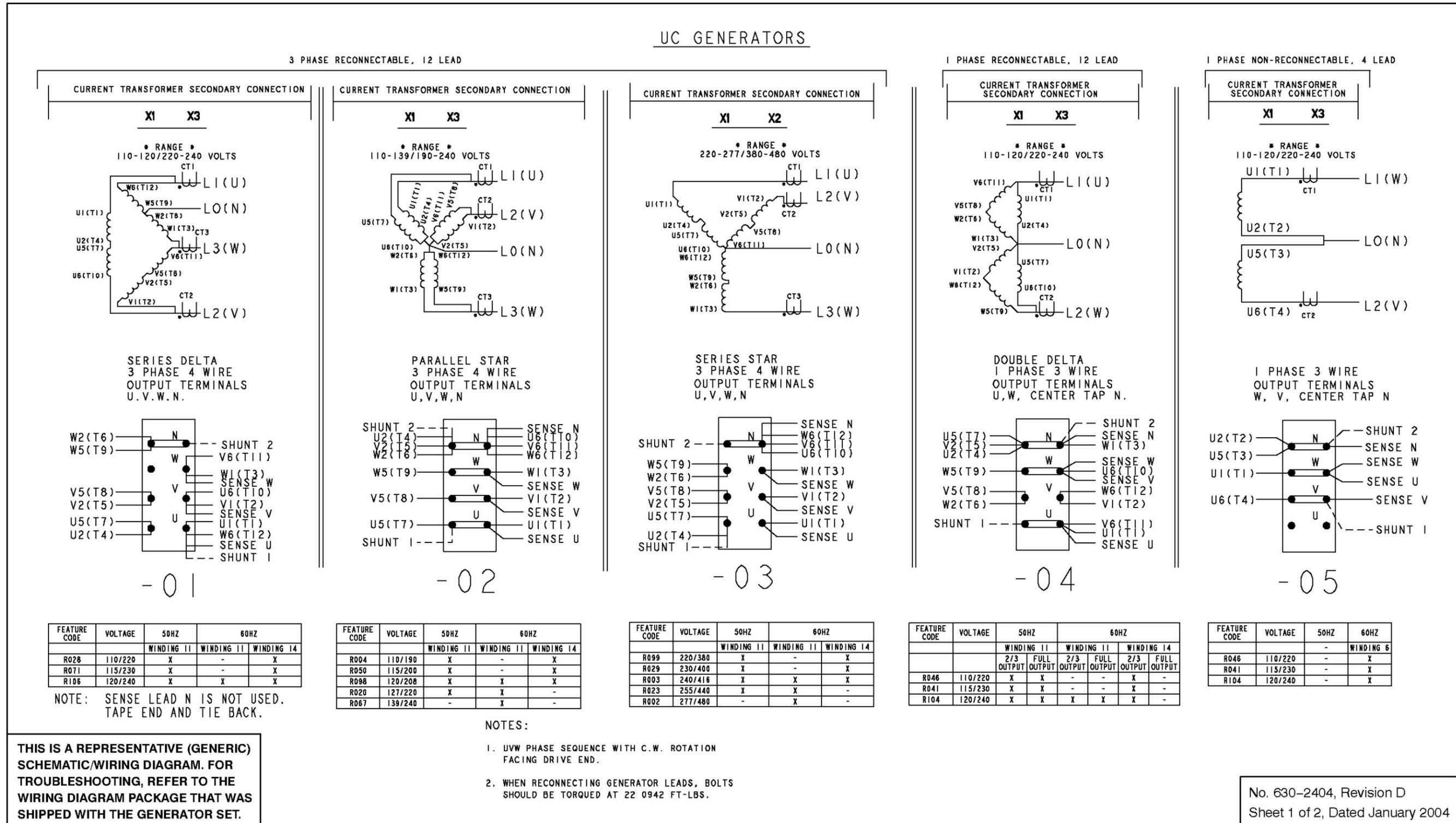
FIGURE 41. ALTERNATOR RECONNECT DRAWING 630-2402 SHEET 1
