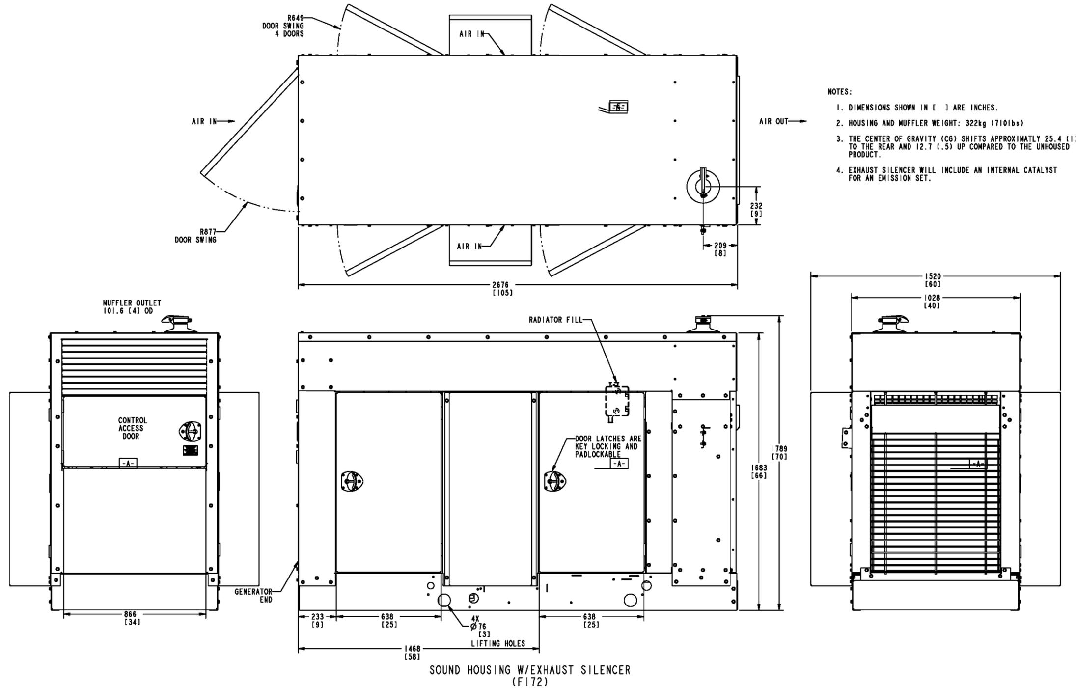
FIGURE 39. OULINE DRAWING - SOUND HOUSED WITH EXHAUST (F172)
