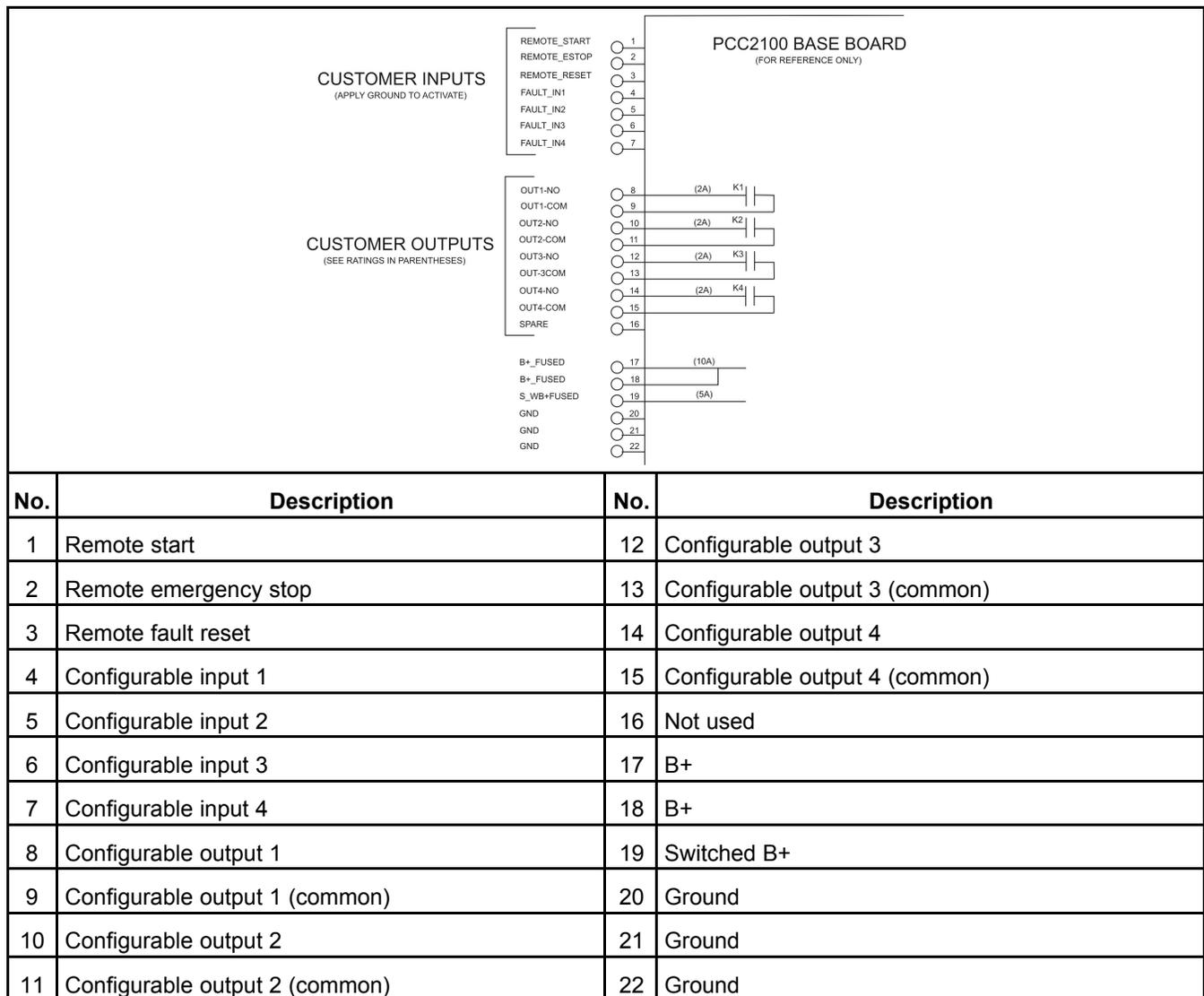
FIGURE 19. PCC 2100 TB1 CUSTOMER CONNECTIONS
