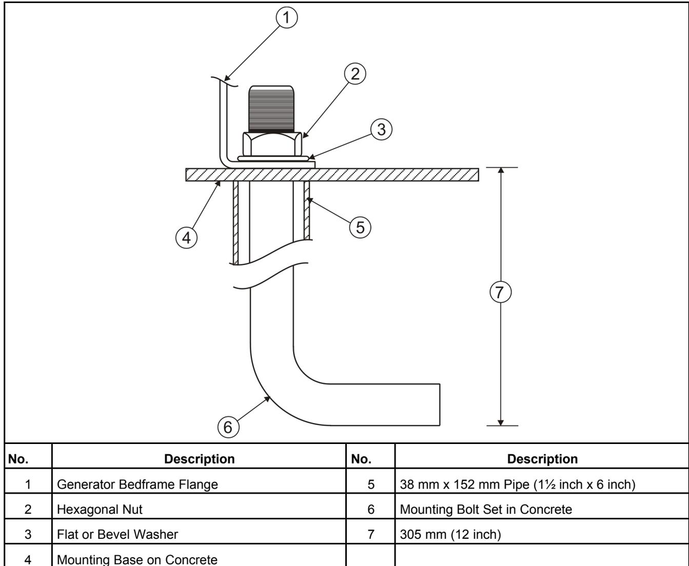
FIGURE 7. BOLT DIAGRAM
