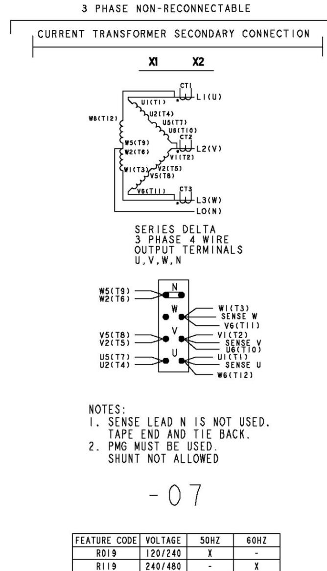
FIGURE 42. ALTERNATOR RECONNECT DRAWING - 630-2404 SHEET 2
