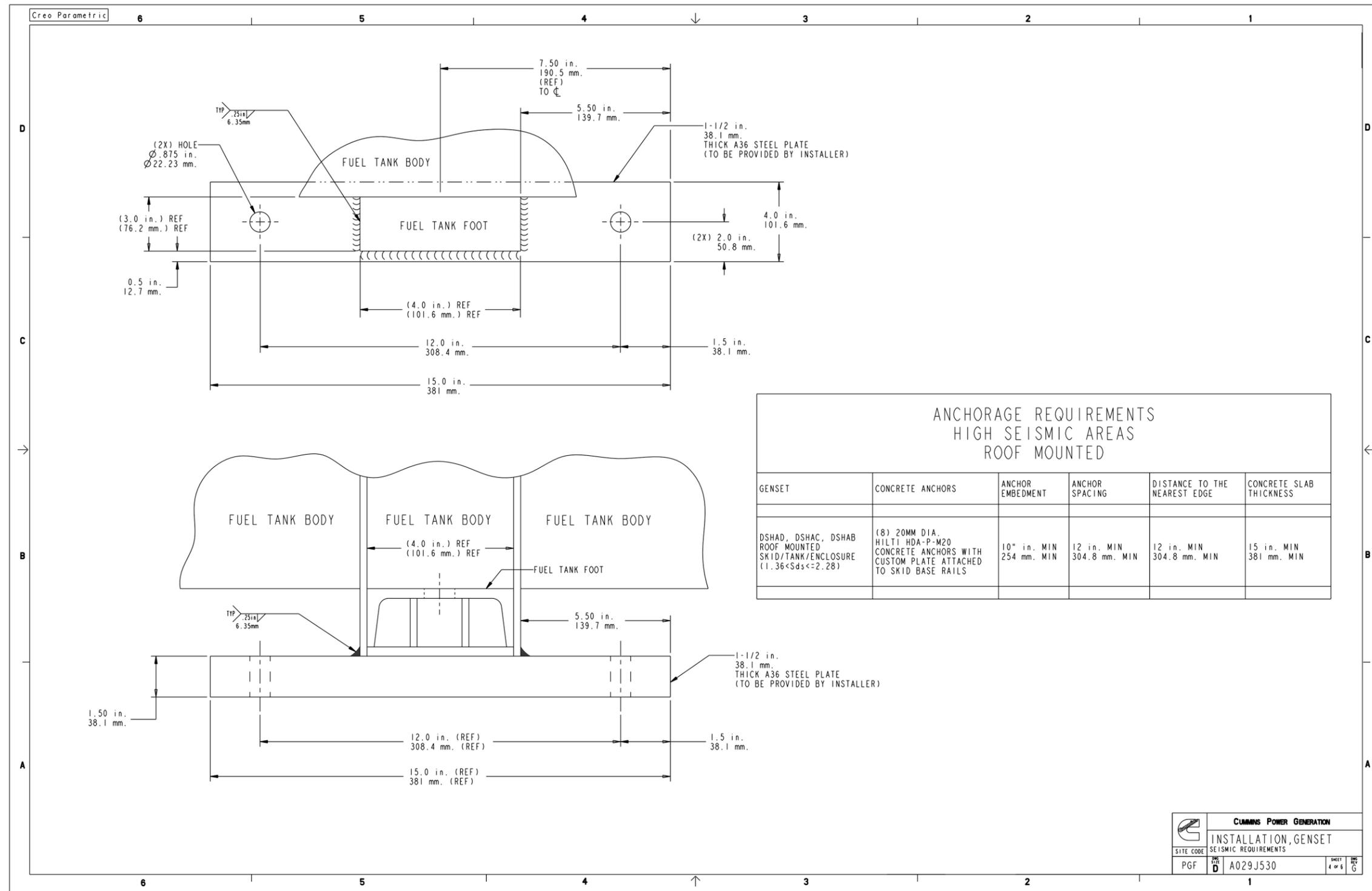
FIGURE 46. SEISMIC INSTALLATION INSTRUCTIONS (SHEET 4 OF 5)
