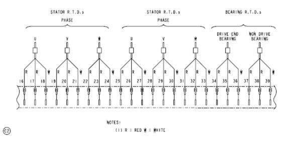
FIGURE 37. CUSTOMER CONNECTIONS DRAWING - 620-0247 SHEET 2
