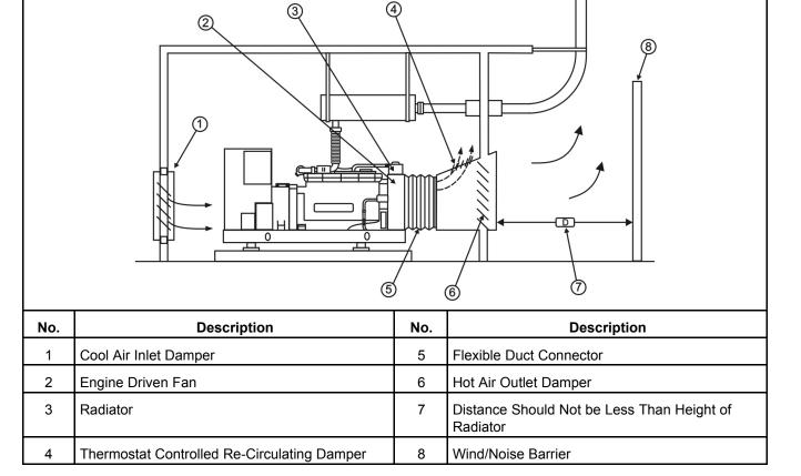
FIGURE 18. TYPICAL OPEN GENERATOR SET INSTALLATION
