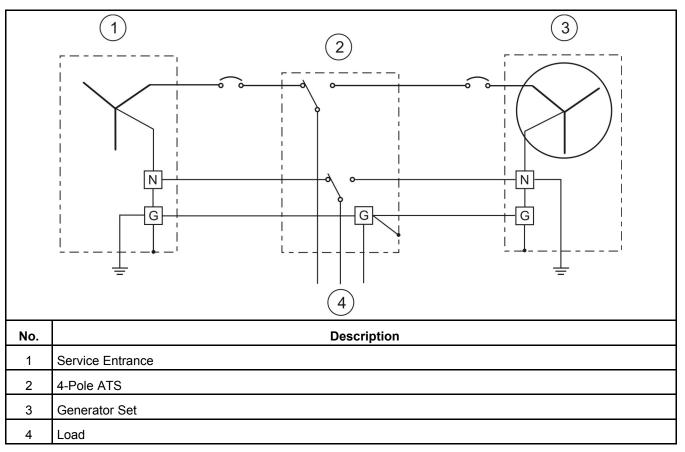
FIGURE 31. TYPICAL SYSTEM - THREE-PHASE, FOUR WIRE UTILITY, FOUR-POLE ATS
