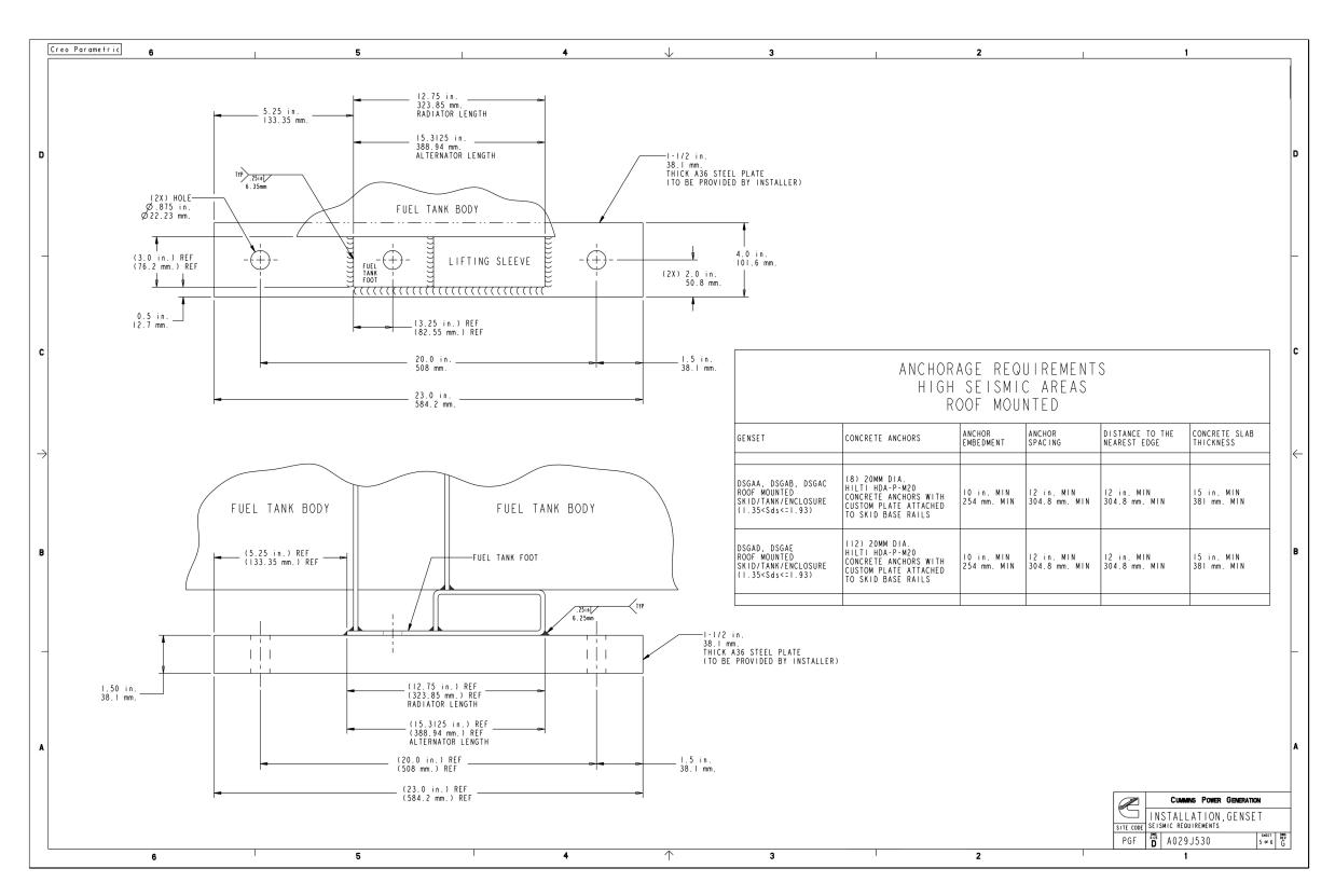
FIGURE 47. SEISMIC INSTALLATION INSTRUCTIONS (SHEET 5 OF 5)
