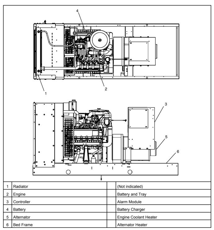
FIGURE 2. TYPICAL FORD V-10 6.8L ENGINE GENERATOR SET
