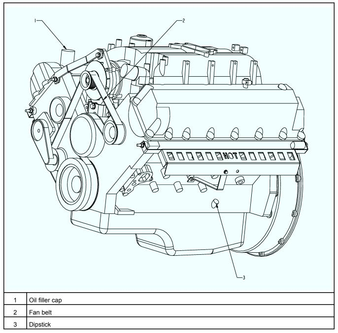
FIGURE 3. TYPICAL ENGINE COMPONENTS (FORD V-10 6.8L)
