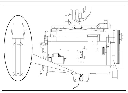
FIGURE 26. OIL PAN HEATER USED IN 120V AND 208/240V APPLICATIONS
