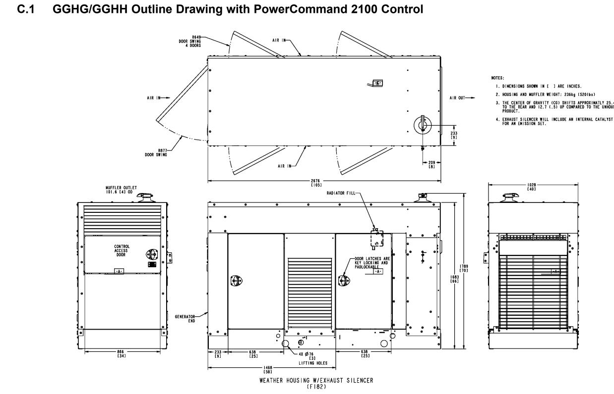
FIGURE 38. OUTLINE DRAWING - WEATHER HOUSED WITH EXHAUST (F182)
