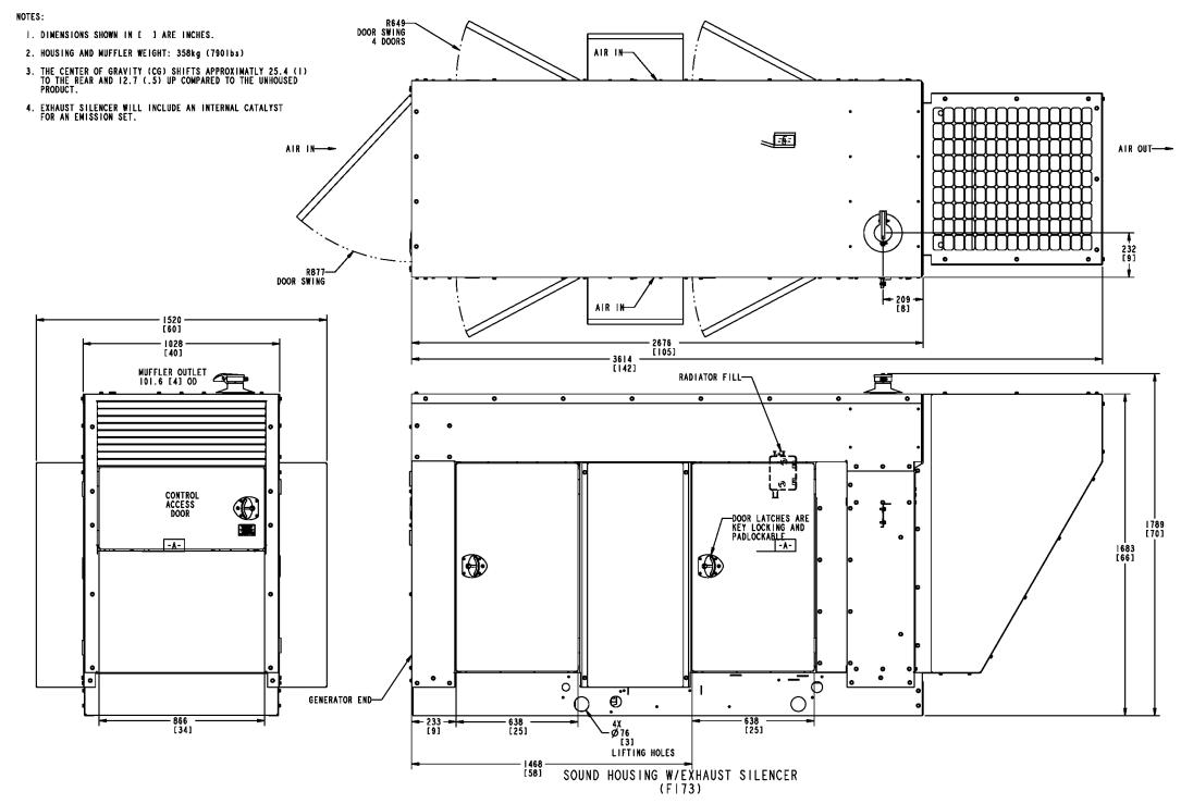
FIGURE 40. OUTLINE DRAWING - SOUND HOUSED WITH EXHAUST (F173)
