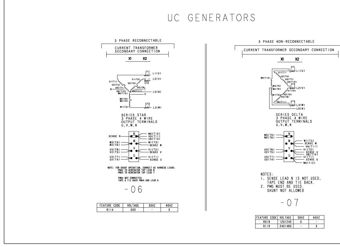
FIGURE 42. ALTERNATOR RECONNECT DRAWING - 630-2404 SHEET 2
