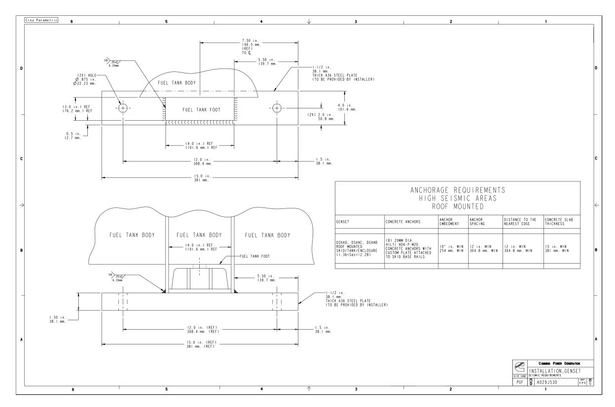
FIGURE 46. SEISMIC INSTALLATION INSTRUCTIONS (SHEET 4 OF 5)
