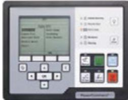
**PowerCommand 2.3 control** - An integrated generator set control system providing voltage regulation, engine protection, generator protection, operator interface, and isochronous governing (optional).
