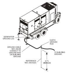
If used as an alternate power supply, connect only after the main service entrance switch has been DISCONNECTED and LOCKED OPEN. In addition, circuit overload protection must be provided in accordance with National Electrical Codes and local regulations.
