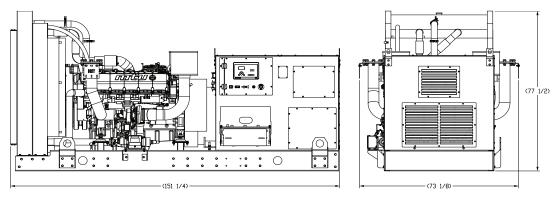
Drawing above for illustration purposes only, based on standard open power 480 volt engine-generator set. Lengths may vary with other voltages. Do not use for installation design. See website for unit specific template drawings.
