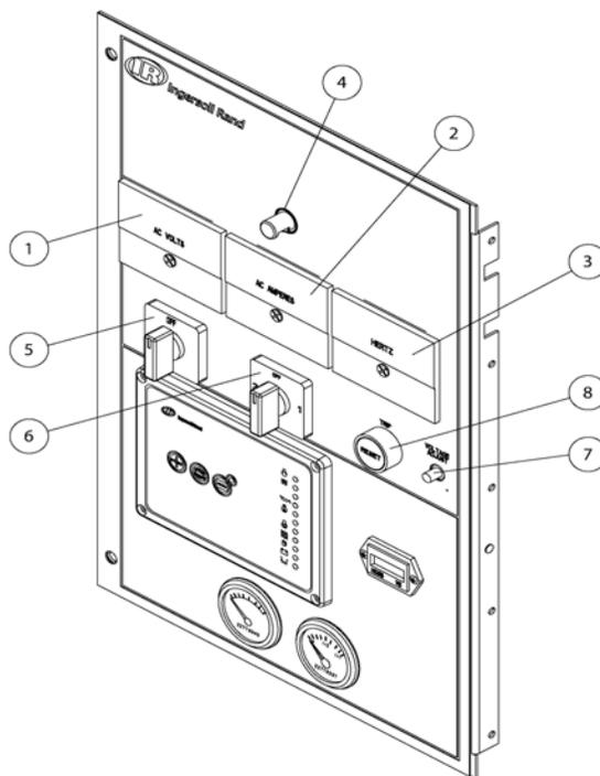
**CIRCUIT BREAKERS - Flip to Reset (if equipped)**
